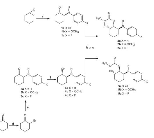
Scheme 1. Synthesis route for isomers *cis* and *trans*-2-arylaminocyclohexyl *N*,*N*-dimethylcarbamates. Reagents and conditions: (a) arylamine, H<sub>2</sub>O, 60 °C, 48 h; (b) Na°/THF, 80 °C, 8 h; *N*,*N*-dimethylcarbamoyl chloride, reflux, 16 h; (c) NaH/THF, 80 °C, 8 h; *N*,*N*-dimethylcarbamoyl chloride, reflux, 16 h; (d) Br<sub>2</sub>, H<sub>2</sub>O, 0-5 °C; (e) Na<sub>2</sub>CO<sub>3</sub>, quinoline, methoxyethanol, reflux, 2 h; and (f) *N*-selectride, THF, –78 °C, 4 h.
