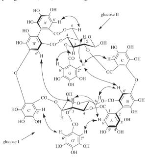
**Figure 3**. Through-space <sup>1</sup>H-<sup>1</sup>H correlations determined by the NOESY experiment.
