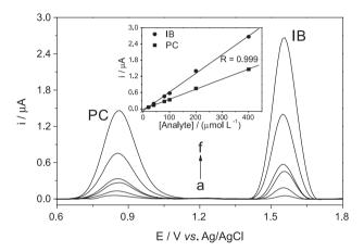
**Figure 5.** DPVs in 0.1 mol  $L^{-1}$  H<sub>2</sub>SO<sub>4</sub> over a BDD electrode containing PC and IB in the following concentrations (µmol  $L^{-1}$ ): 20 (a); 40 (b); 80 (c); 100 (d); 200 (e); and 400 (f). The respective calibration curves, including the correlation coefficient, are shown in the inset. DPV conditions: amplitude: 50 mV; pulse time: 500 ms; pulse width: 10 mV; scan rate: 20 mV s<sup>-1</sup>.
