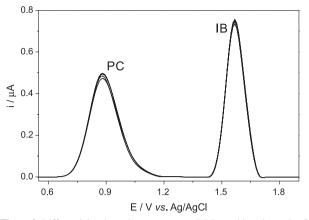
**Figure 2.** Differential-pulse voltammograms at BDD working electrode of the supporting electrolyte plus 0.1 mmol  $L^{-1}$  PC and IB. DPV conditions: amplitude: 50 mV; pulse time: 500 ms; pulse width: 10 mV; scan rate: 20 mV s<sup>-1</sup>.
