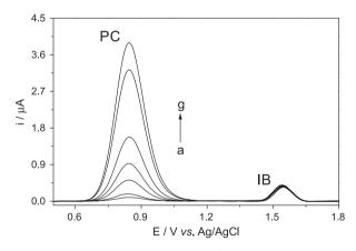
**Figure 3.** DPV over BDD in 0.1 mol  $L^{-1}$  H<sub>2</sub>SO<sub>4</sub>. IB with constant concentration at 50 µmol  $L^{-1}$  and changing PC concentration of 20 (a) up to 800 (g) µmol  $L^{-1}$ . DPV conditions: amplitude: 50 mV; pulse time: 500 ms; pulse width: 10 mV; scan rate: 20 mV s<sup>-1</sup>.
