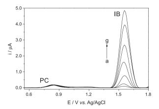
**Figure 4.** DPV over BDD in 0.1 mol  $L^{-1}$  H<sub>2</sub>SO<sub>4</sub>. PC with constant concentration at 50 µmol  $L^{-1}$  and changing IB concentration of 20 (a) up to 800 (g) µmol  $L^{-1}$ . DPV conditions: amplitude: 50 mV; pulse time: 500 ms; pulse width: 10 mV; scan rate: 20 mV s<sup>-1</sup>.
