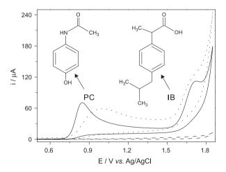
**Figure 1.** Cyclic voltammograms of the supporting electrolyte 0.1 mol  $L^{-1}$  H<sub>2</sub>SO<sub>4</sub> with 10% (v/v) ethanol (---) plus the addition of 1.0 mmol  $L^{-1}$  PC and IB 1.0 mmol  $L^{-1}$  at the BDD working electrode after anodic (—) and cathodic (…) pretreatment. Scan rate: 50 mV s<sup>-1</sup>. The chemical structures of PC and IB are shown in the inset.
