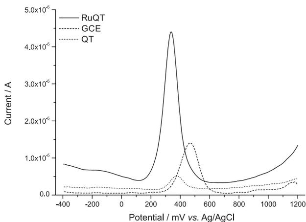
**Figure 11.** Electrochemical comparison among RuQT, QT and GCE electrodes in acetaminophen analyses, in pH 1.0.
