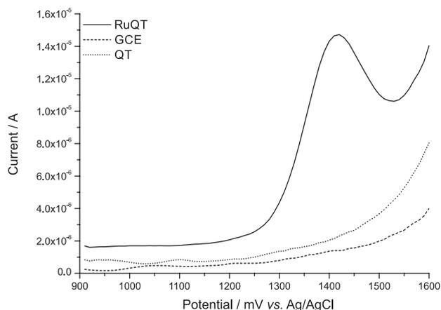
**Figure 6.** Electrochemical comparison among RuQT, QT and GCE electrodes in the analysis of sildenafil citrate, in pH 1.0.
