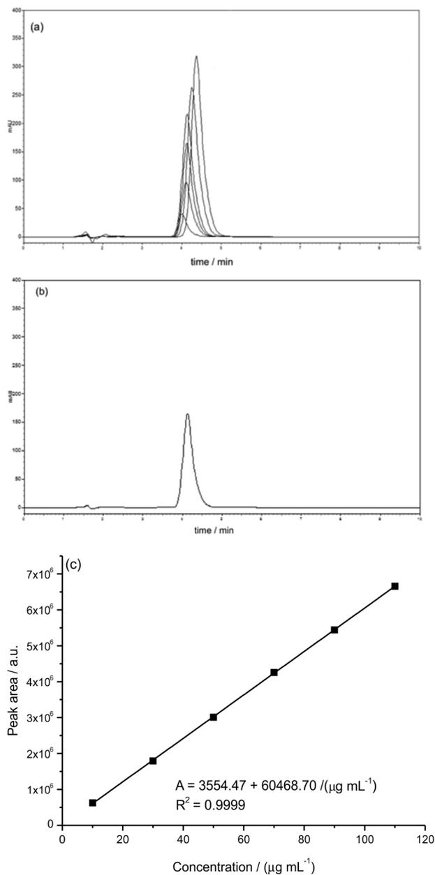
**Figure 15.** (a) Chromatograms of sildenafil citrate; (b) commercial drug analysis; (c) calibration curve for sildenafil citrate.
