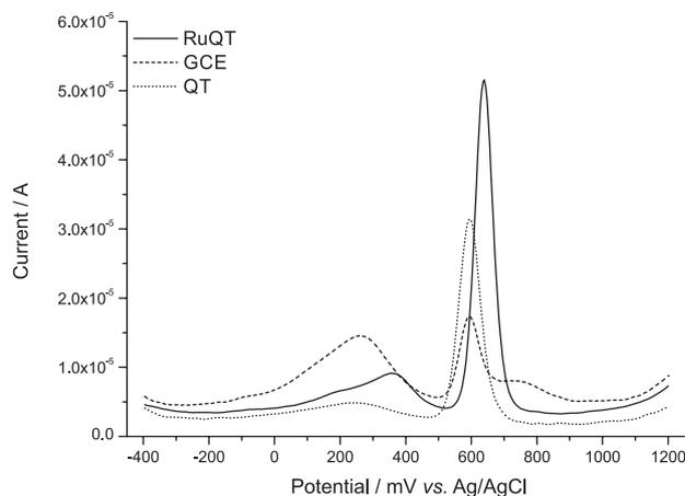
**Figure 12.** Electrochemical comparison among RuQT, QT and GCE electrodes in acetaminophen analyses, in pH 6.5.
