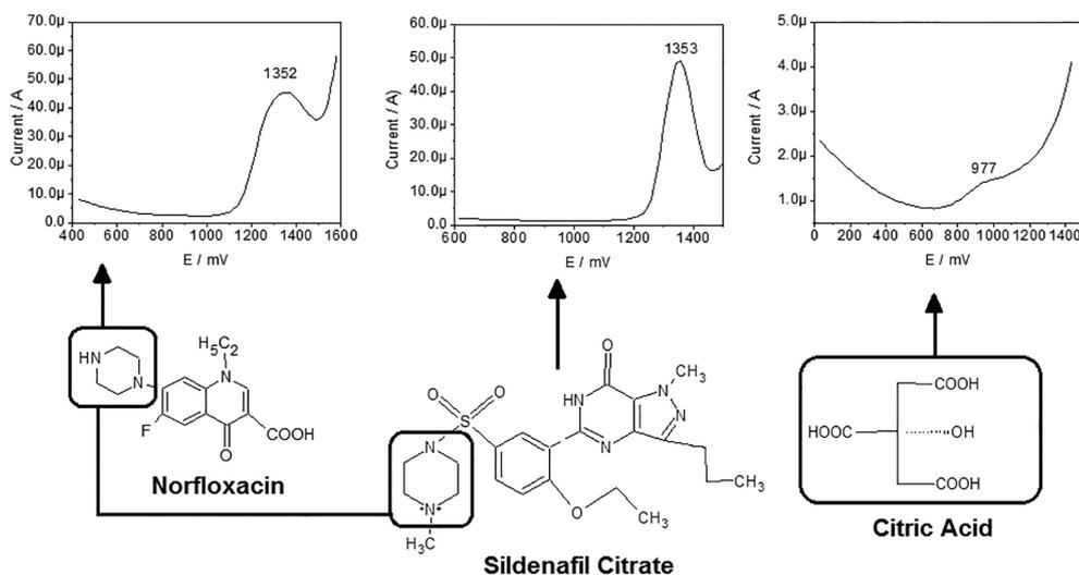
**Figure 7.** Electrochemical oxidation of three different compounds: norfloxacin; sildenafil citrate and citric acid, in  $0.1 \text{ mol L}^{-1} \text{ H}_2\text{SO}_4$  electrolyte.
