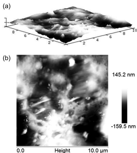
**Figure 4.** AFM pictures of the film surface: (a) in 3D and (b) in 2D, 10  $\mu$ m<sup>2</sup> area.
