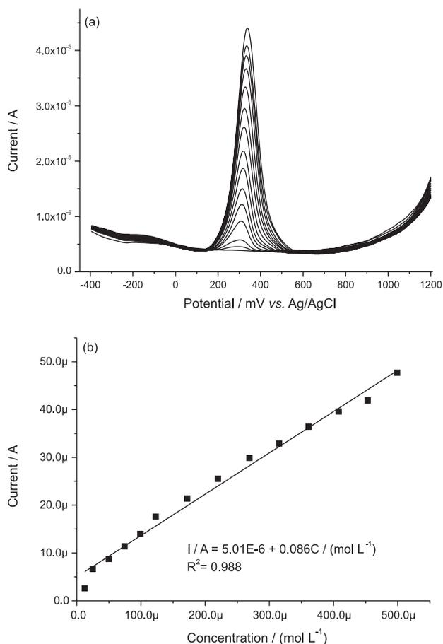
**Figure 9.** (a) DPV of acetaminophen - RuQT electrode oxidation - pH 1.0 ( $1.25 \times 10^{-5}$  to  $4.99 \times 10^{-4} \text{ mol L}^{-1}$ ); (b) analytical curve of acetaminophen in pH 1.0.
