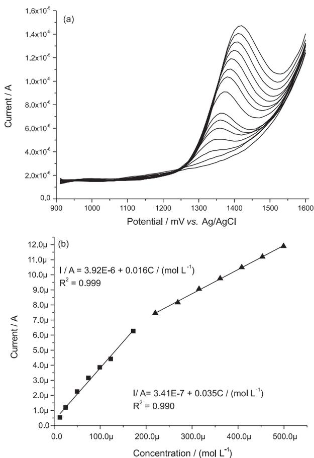
**Figure 5.** (a) DPV of sildenafil citrate - RuQT electrode oxidation - pH 1.0 ( $1.25 \times 10^{-5}$  to  $4.99 \times 10^{-4}$  mol L<sup>-1</sup>); (b) analytical curves of sildenafil citrate in pH 1.0 where the first curve is  $1.25 \times 10^{-5}$  to  $1.72 \times 10^{-4}$  mol L<sup>-1</sup> and the second curve is  $2.20 \times 10^{-4}$  to  $4.99 \times 10^{-4}$  mol L<sup>-1</sup>.
