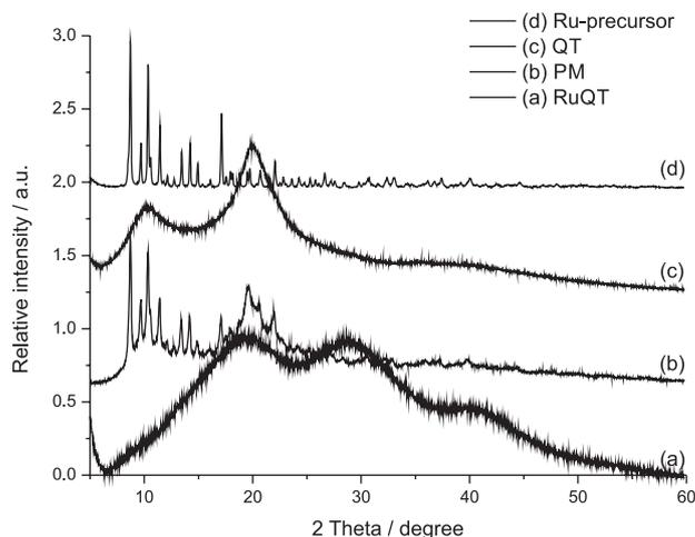
**Figure 3.** Comparison of powder XRD of RuQT compound (a), a PM containing Ru-precursor and free QT (b), free QT (c) and the precursor *mer*-[RuCl<sub>3</sub>(dppb)H<sub>2</sub>O] (d).
