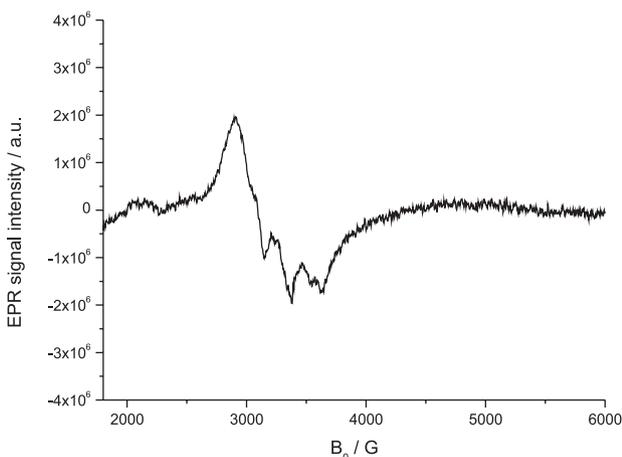
**Figure 2.** EPR spectrum of RuQT at 77 K in solid state.
