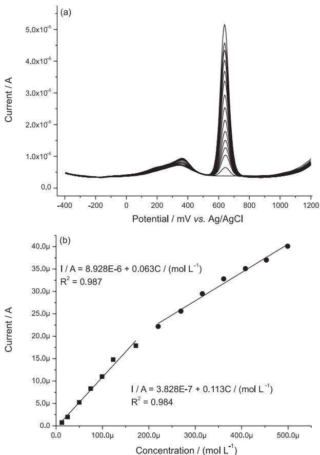
**Figure 10.** (a) DPV of the acetaminophen - RuQT electrode oxidation - pH 6.5 ( $1.25 \times 10^{-5}$  to  $4.99 \times 10^{-4}$  mol L $^{-1}$ ); (b) analytical curves of acetaminophen in pH 6.5 where the first curve is  $1.25 \times 10^{-5}$  to  $1.72 \times 10^{-4}$  mol L $^{-1}$  and the second curve is  $2.20 \times 10^{-4}$  to  $4.99 \times 10^{-4}$  mol L $^{-1}$ .
