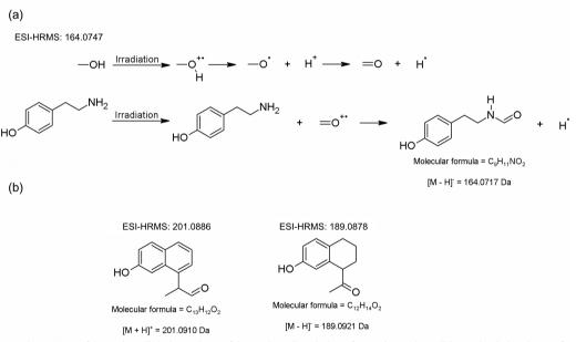
Figure 5. (a) Proposed structures of the main radiolytic products of the methanolic solution of tyramine and possible mechanistic schemes for their formation and (b) proposed structures of the radiolytes of tyramine irradiated in aqueous solution according to the exact mass encountered.
