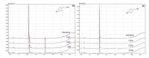
**Figure S3.** Chromatograms of the methanolic (A) and aqueous (B) solutions of tyramine after irradiation at different doses. Mode: scan; Column: RTX-5MS (5% diphenyl/95% dimethyl polysiloxane); Ramp: 2 min, 80 °C; 10 °C min<sup>-1</sup>, 80 °C to 280 °C.
