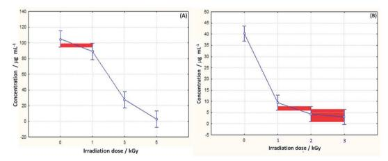
Figure S2. Plot of the phenylethylamine concentration vs. irradition dose for the methanolic solutions (A) and the aqueous solutions (B).
