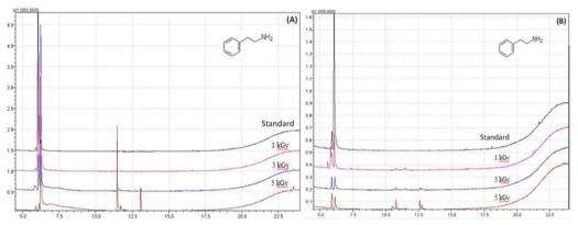
**Figure S1.** Chromatograms of the methanolic (A) and aqueous (B) solutions of phenylethyamine after irradiation at different doses. Mode: scan; Column: RTX-5MS (5% diphenyl/95% dimethyl polysiloxane); Ramp: 2 min, 80 °C; 10 °C min<sup>-1</sup>, 80 °C to 280 °C.
