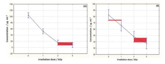
Figure S4. Plot of the tyramine concentration vs. irradition dose for the methanolic solutions (A) and the aqueous solutions (B).
