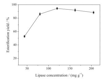
**Figure 4.** The effect of concentration of lipase on esterification in DBSA microemulsion system (reaction conditions: molar ratio (alcohol/acid) 4,  $w_0$  3.3, time 4 h).
