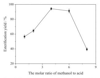
**Figure 2.** Effect of molar ratio on esterification catalyzed by CRL in DBSA microemulsion system (reaction conditions:  $w_0$  3.3, time 4 h, lipase 120 mg g<sup>-1</sup>).
