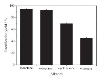
**Figure 5.** Effect of different kinds of microemulsion system on esterification (reaction conditions:molar ratio (alcohol/acid) 4,  $w_0$  3.3, time 4 h, lipase 120 mg g<sup>-1</sup>).
