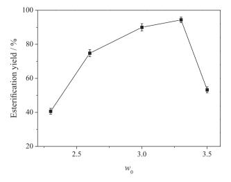
**Figure 1.** Effect of  $w_0$  on esterification catalyzed by CRL in DBSA microemulsion system (reaction conditions: molar ratio (alcohol/acid) 4, time 4 h, lipase 120 mg g<sup>-1</sup>).
