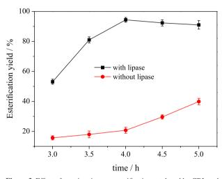
**Figure 3.** Effect of reaction time on esterification catalyzed by CRL and without CRL in DBSA microemulsion system (reaction conditions: molar ratio (alcohol/acid) 4,  $w_0$  3.3, lipase 120 mg g<sup>-1</sup>).
