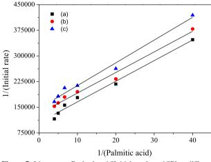
**Figure 7.** Lineweaver-Burk plot: 1/[Initial rate] vs. 1/[P] at different concentration of methanol, (a)  $0.2 \text{ mol } L^{-1}$ ; (b)  $0.25 \text{ mol } L^{-1}$ ; (c)  $0.3 \text{ mol } L^{-1}$ .
