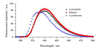
**Figure 3.** Emission spectra recorded to the quinoline **8b** in acetonitrile ( $\Box$ ), ethanol ( $\bullet$ ) and cyclohexane ( $\triangle$ ).  $\lambda_{exc} = 350$  nm.
