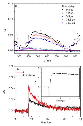
**Figure 6.** (a) Transient absorption spectrum for **8d** in the presence of phenol  $(1 \times 10^{-4} \text{ mol } \text{L}^{-1})$  and (b) transient decay of **8d** in the presence and absence of phenol at 390 nm. Inset: growth and decay lifetime of **8d** + phenol solution monitored at 390 nm on a short timescale.
