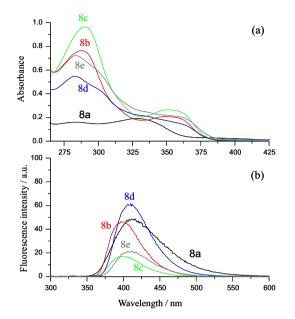
Figure 2. Absorption (a) and fluorescence (b) spectra of quinolines 8a-e in dichloromethane (DCM);  $\lambda_{esc} = 350$  nm.
