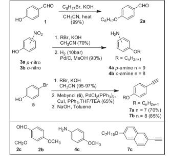
Scheme 1. Preparation of key intermediates 2a, 4a and 7a-b.
