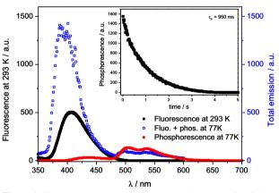
Figure 4. Fluorescence and phosphorescence emission (total emission) of 8d in ethanol at 77 K (blue dots) and fluorescence emission at 293 K (black dots). Insert demonstrates the phosphorescence time decay at 77 K.
