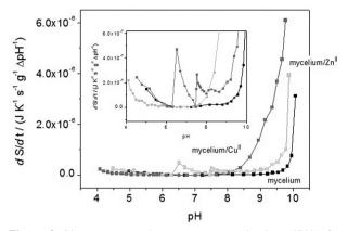
**Figure 8.** Slow-proton exchange entropy production (dS/dt) for out-of-equilibrium processes during titration for the [mycelium/metal ion/ water] complex systems. [mycelium], [mycelium/Zn<sup>II</sup>] and [mycelium/ Cu<sup>II</sup>] complex systems are represented by black, gray and light gray lines respectively. Entropy production values are normalized with respect to pH variation between sequential titration points ( $\Delta pH^{-1}$ ) and mycelium mass (g<sup>-1</sup>).
