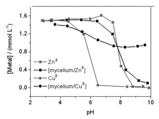
**Figure 4.** Metal ion ( $Zn^{II}$  and  $Cu^{II}$ ) concentrations in soluble/suspension phase (filtered < 0.2 µm) at pH 2-10 for [metal ion/water] and [mycelium/ metal ion/water] complex systems.
