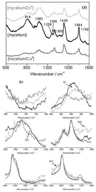
**Figure 3.** In (a) [mycelium] and [mycelium/metal ion] Raman spectra. In (b) composite figure of [mycelium] and [mycelium/metal ion] enlarged spectra. [mycelium], [mycelium/Cu<sup>II</sup>] and [mycelium/Zn<sup>II</sup>] are represented in black, gray and light gray lines, respectively.
