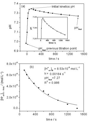
**Figure 2.** Example of (a) out-of-equilibrium pH stabilization measurement from pH<sub>final</sub> of the previous titration point to pH<sub>final</sub> of actual titration point (passing through (*i*) fast and (*ii*) slow proton exchange) and (b) first order kinetic plot for the [mycelium/Cu<sup>II</sup>/water] system at pH<sub>final</sub> 7.27 (plot construction and derivation of  $[H^+_{ex}]_{i0}$  and k are detailed in out-of-equilibrum modeling section).
