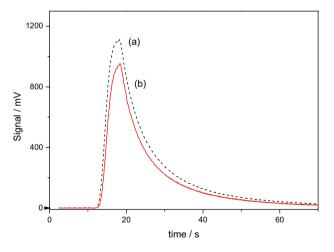
Figure 3. Records of the luminometer readout. Curves (a) and (b) are signals generated using a blank solution and a 0.6 mg mL<sup>-1</sup> folic acid solution, respectively.
