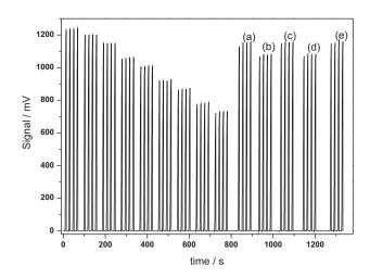
**Figure 7.** Records of the luminometer readout. From left folic acid standard solution 0.0, 0.1, 0.2, 0.5, 0.7, 1.0, 1.3, 1.7 and 2.0 mg mL<sup>-1</sup>; followed of five folic acid samples.
