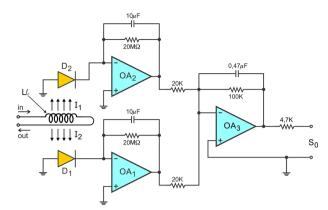
**Figure 1.** Diagram of the luminometer.  $D_1$  and  $D_2$  = photodiodes;  $OA_1$ ,  $OA_2$  and  $OA_3$  = operational amplifiers OP07;  $S_0$  = generated signal (mV);  $I_1$  and  $I_2$  = radiation beams emanated from the reaction coil; Ll = chemiluminescence reaction coil.
