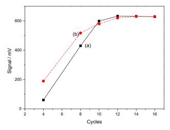
**Figure 4.** Effect of the sampling cycles. Curves (a) and (b) correspond to the variation of sample and luminol solution inserting cycles, respectively, achieved using a 1.0 mmol  $L^{-1}$  luminol solution prepared in a 0.4 mol  $L^{-1}$  NaOH medium and a 20 mmol  $L^{-1}$  hexacyanoferrate(III) solution.
