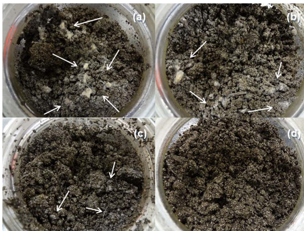
Figure 7. Interior of jars after 60 days of DMR experiments: (a) pristine cassava starch; (b) TPS; (c) Star/Vee-Chit 5.0%; (d) control.
