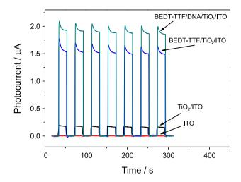
**Figure 1.** Photocurrent response of BEDT-TTF/DNA/TiO<sub>2</sub>/ITO, BEDT-TTF/TiO<sub>2</sub>/ITO, TiO<sub>2</sub>/ITO, and ITO. Experiments carried in 0.1 phosphate buffer solution (pH 7.0) containing 1 mmol L<sup>-1</sup> adrenaline.  $E_{aop} = 0.25 V vs. Ag/AgCl.$
