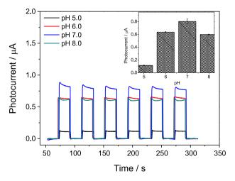
**Figure 4.** Influence of pH of the solution on the photosensor response for 100 µmol L<sup>-1</sup> adrenaline. Measurements were carried out in 0.1 mol L<sup>-1</sup> phosphate buffer solution.  $E_{app} = 0.25$  V vs. Ag/AgCl.
