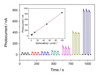
**Figure 6.** Photocurrent of photoelectrochemical sensor obtained under optimized conditions to adrenaline concentrations between 0.01 and  $100 \mu$ mol L<sup>-1</sup>. Inset: analytical curve.
