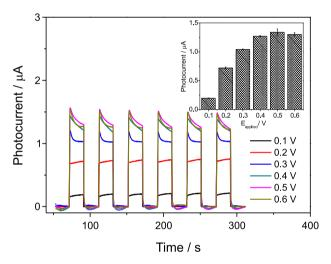
**Figure 5.** Influence of applied potential on the photocurrent for  $100 \,\mu\text{mol}\,\text{L}^{-1}$  of adrenaline. Measurements were carried out in 0.1 mol  $\text{L}^{-1}$  phosphate buffer solution.
