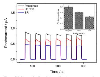
**Figure 3.** Influence of buffer solution on the photosensor response for 100  $\mu$ mol L<sup>-1</sup> of adrenaline. Measurements were carried out in 0.1 mol L<sup>-1</sup> phosphate buffer solution. E<sub>app</sub> = 0.25 V *vs.* Ag/AgCl.
