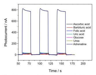
**Figure 7.** Photocurrent obtained for proposed photoelectrochemical sensor toward several foreign species in comparison to that obtained for adrenaline under optimized conditions at an applied potential of 0.4 V *vs.* Ag/AgCl. The concentration of all species was fixed at 100 µmol L<sup>-1</sup>.
