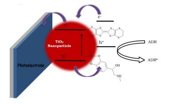
Figure 2. Proposed mechanism for the photoelectrochemical detection of adrenaline.
