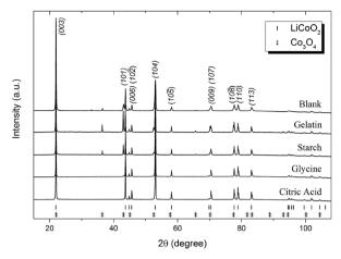
Figure 4. Powder X-ray pattern of the samples prepared from the citric acid, glycine, starch, gelatin precursors and the blank test.
