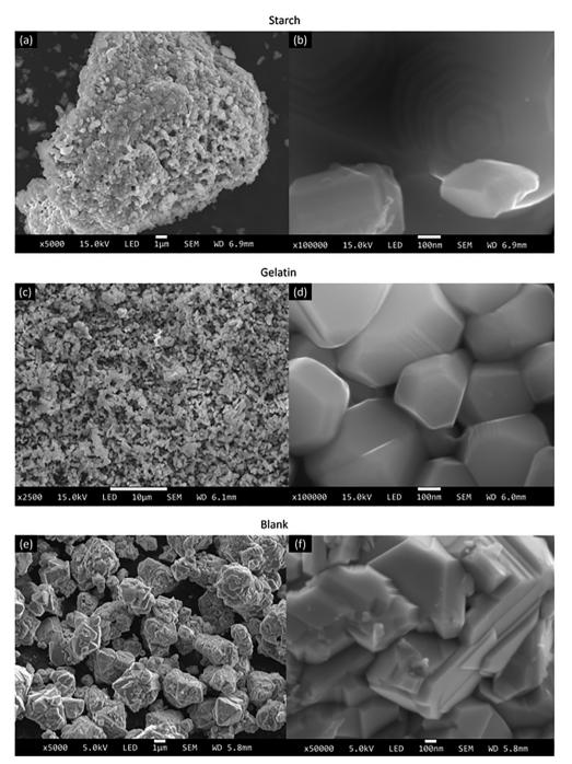
Figure 10. SEM of the synthesized HT-LiCoO<sub>2</sub> samples with the starch and gelatin precursors and the blank test, expanded at  $5000\times$  (a and e),  $100000\times$  (b and d),  $50000\times$  (f) and  $2500\times$  (c).
