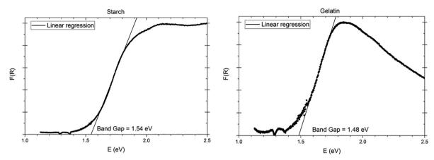
Figure 7. DRS, Kubelka-Munk function, F(R), and tangent line extrapolation. Results for the starch (left) and gelatin (right) samples.
