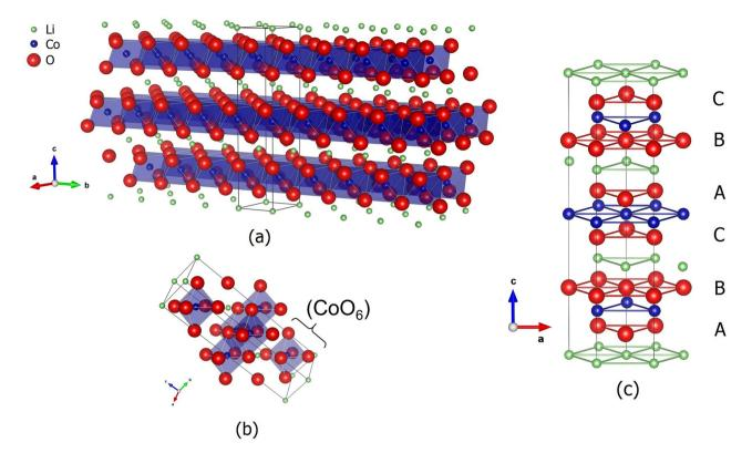
Figure 1. (a) Layered crystalline structure of the rhombohedral  $LiCoO_2$ ; (b) representation of the octahedral  $CoO_6$  structure; (c) stacking arrangement of the layers (ABCABC).
