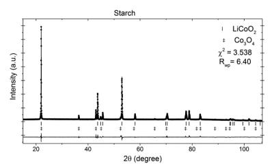
Figure 5. Rietveld refinement, using the symmetry  $R\overline{3}m$ , for sample of HT-LiCoO<sub>2</sub> obtained with the starch precursor. The bottom line shows the difference between the experimental and calculated result.
