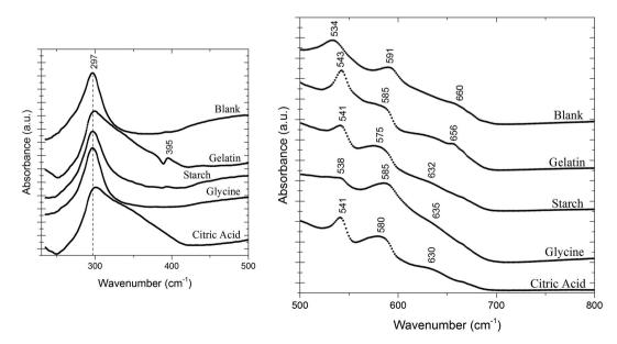
Figure 2. FTIR absorption spectra of  $LiCoO_2$  in the low (left side) and high (right side) wavenumber regions, for all complexing agents used in the synthesis and for the blank test.
