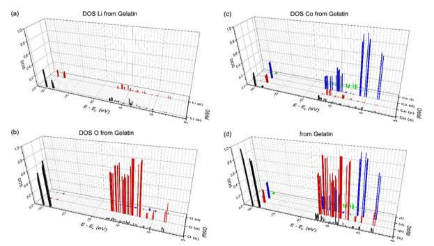
Figure 8. DOS for the  $LiCoO_2$  in each orbital obtained from gelatin for: (a)  $Li^*$ , (b)  $Co^{3*}$ , (c)  $O^{2*}$  and (d) density of total states. The energy value at zero corresponds to the Fermi level, negative values near zero correspond to valence band and positive values near zero correspond to the conduction band.
