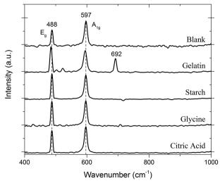
Figure 3. Raman spectra of the samples of  $HT-LiCoO_2$  synthesized with the four complexing agents and the blank test.
