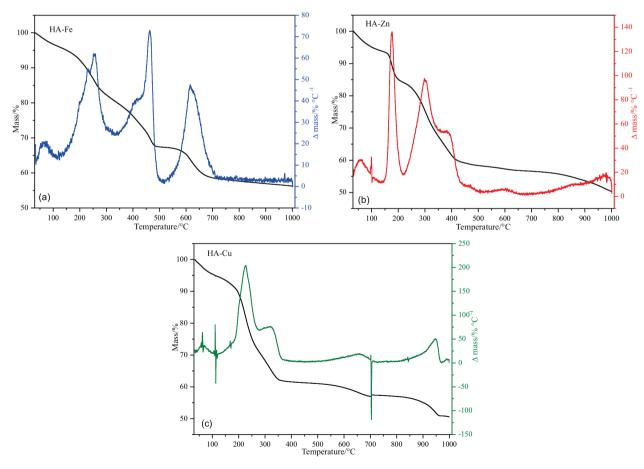
Figure 8. Thermogravimetry: TG and DTG curves of humic acid complex (a) with iron (HA-Fe); (b) with zinc (HA-Zn); (c) with copper (HA-Cu).
