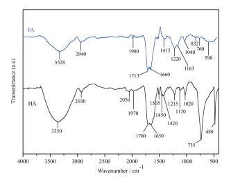
Figure 1. FTIR spectra of humic acid (HA) and fulvic acid (FA).
