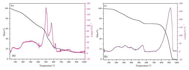
Figure 7. Thermogravimetry: TG and DTG curves of (a) humic acid (HA); (b) fulvic acid (FA).
