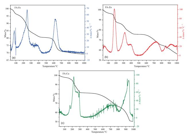
Figure 9. Thermogravimetry: TG and DTG curves of fulvic acid complex (a) with iron (FA-Fe); (b) with zinc (FA-Zn); (c) with copper (FA-Cu).
