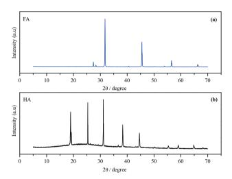
Figure 4. X-ray diffraction: diffractogram of (a) fulvic acid; (b) humic acid.
