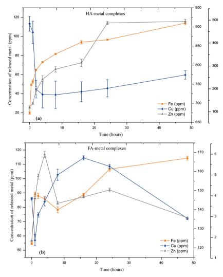
Figure 10. Curves of the release of the humic acid (a) and fulvic acid (b) complexed with the metals: iron, copper and zinc.
