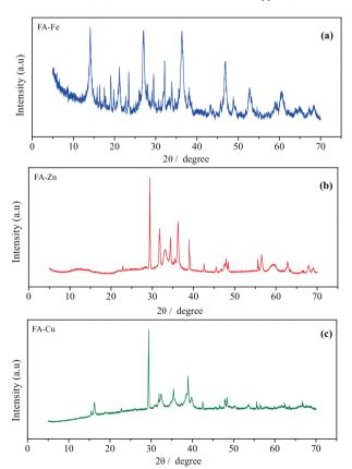
**Figure 6.** X-ray diffraction: diffractogram of complex of fulvic acid (a) with iron (FA-Fe); (b) with zinc (FA-Zn); (c) with copper (FA-Cu).
