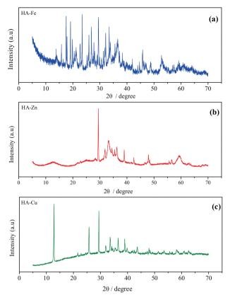
**Figure 5.** X-ray diffraction: diffractogram of complex of humic acid (a) with iron (HA-Fe); (b) with zinc (HA-Zn); (c) with copper (HA-Cu).
