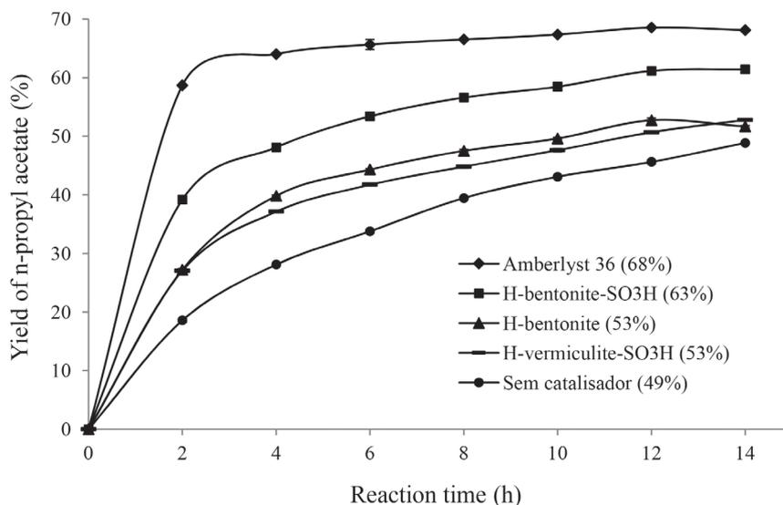
Figure 4. Catalytic performance of catalysts at 100 °C.
