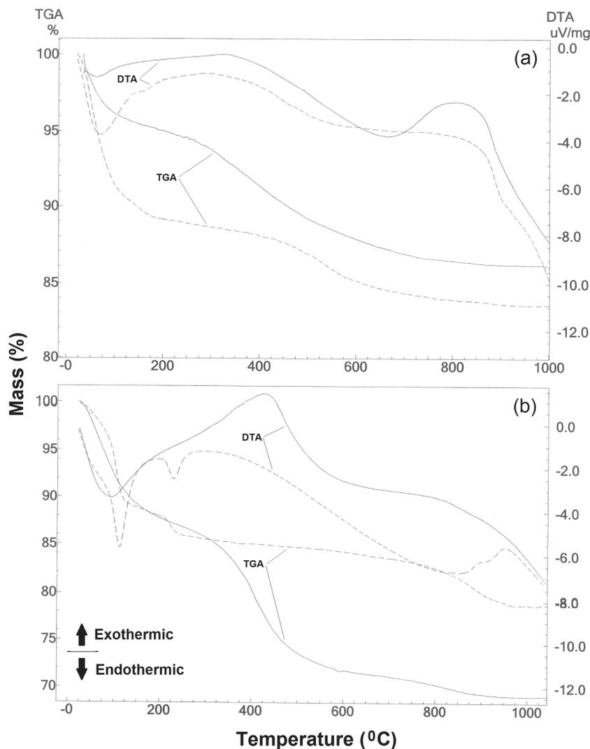
**Figure 2.** TGA curves of the (a) (----) raw bentonite and (—) H-bentonite-SO<sub>3</sub>H samples; (b) (----) raw vermiculite and (—) H-vermiculite-SO<sub>3</sub>H samples.
