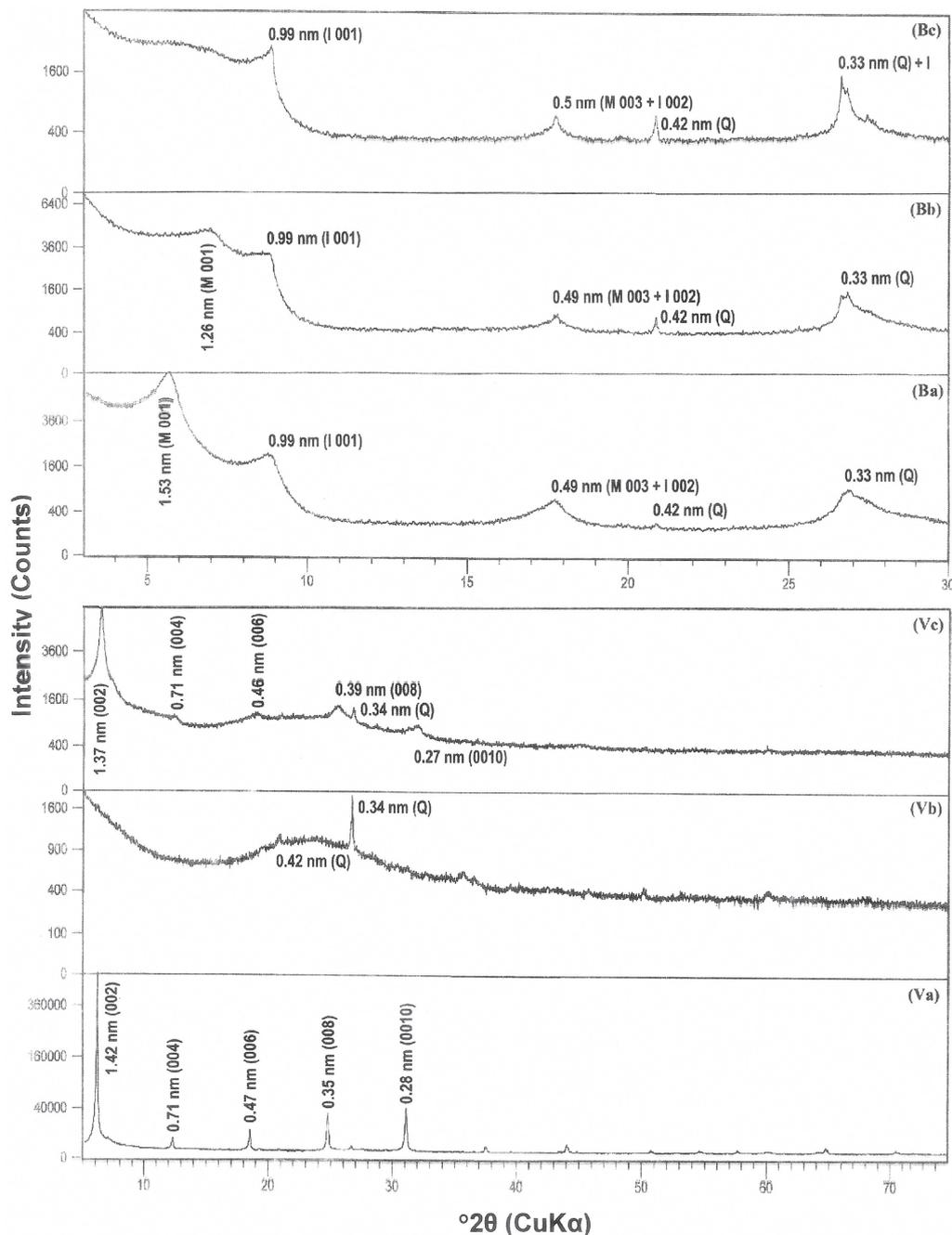
**Figure 1.** X-ray diffraction patterns of the raw bentonite (Ba) and raw vermiculite (Va), H-bentonite (Bb) and H-vermiculite (Vb), H-bentonite-SO<sub>3</sub>H (Bc) and H-vermiculite-SO<sub>3</sub>H (Vc) samples. I: illite, M: montmorillonite, Q: quartz.
