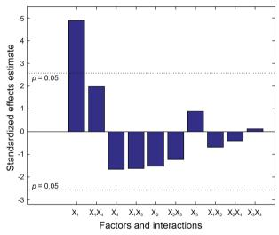
**Figure 2.** Pareto chart for the experiment design II with a horizontal dashed line corresponding to a significance level of p = 0.05, which indicates the solvents mixture significance for the lipids extraction. The symbols are presented in Table 3; X<sub>i</sub>X<sub>j</sub> stands for the interaction between *i* and *j* factors.
