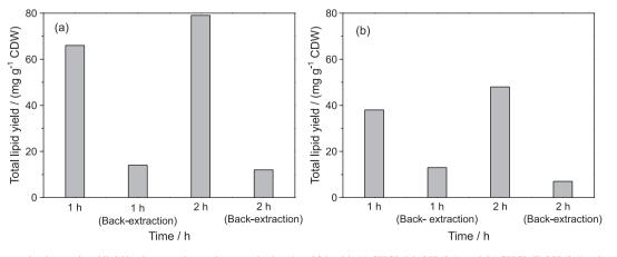
Figure 3. Ultrasonication-assisted lipid back-extraction under water bath at 1 and 2 h with (a) CHCl<sub>3</sub>:MeOH (2:1) and (b) CHCl<sub>3</sub>:EtOH (2:1) solvent mixtures.
