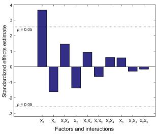
Figure 1. Pareto chart for the experiment design I with a horizontal dashed line corresponding to a significance level of p = 0.05, which indicates the solvents mixture significance for the lipids extraction. The symbols are presented in Table 1; X<sub>i</sub>X<sub>i</sub> stands for the interaction between *i* and *j* factors.
