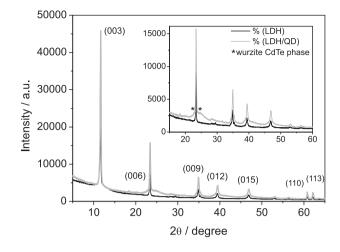
**Figure 1.** X-ray diffraction patterns of LDH and LDH/QD samples. The insertion evidences the region of the crystallographic baseline change between LDH and LDH/QD.
