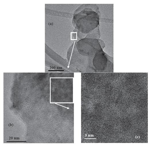
Figure 4. TEM images of LDH/QD sample with different magnifications. (a) Expanded view showing LDH platelets; (b, c) zoom of regions as indicated by the rectangular forms.
