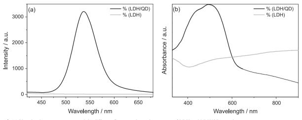
Figure 3. (a) Photoluminescence spectra and (b) diffuse reflectance absorption spectra of LDH and LDH/QD samples.
