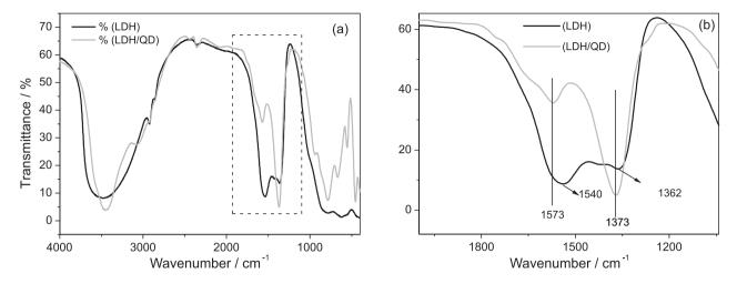
Figure 2. (a) FTIR spectra of LDH and LDH/QD samples; (b) zoom of the region within the rectangle in (a).
