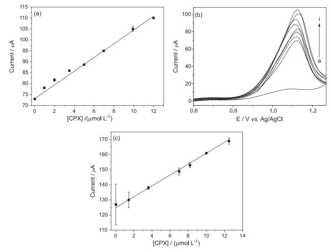
**Figure 6.** (a) Analytical curve obtained from the anodic peak currents for the CPX standard solutions; (b) differential pulse voltammograms obtained with MCPE-LDH/QD in blank solutions and in different CPX concentrations from  $2.5 \times 10^{-8}$  to  $1.2 \times 10^{-5}$  mol L<sup>-1</sup>; (c) analytical curve obtained from the anodic peak currents for the standard addition method used for determination of CPX in commercial tablets.
