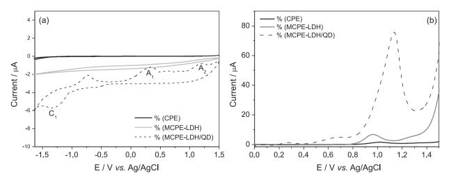
**Figure 5.** (a) Cyclic voltammograms of CPE, MCPE-LDH and MCPE-LDH/QD in phosphate buffer (pH 7.0), scan rate 20 mV s<sup>-1</sup>; (b) differential pulse voltammograms of CPE, MCPE-LDH and MCPE-LDH/QD in the presence of  $5.0 \times 10^{-6}$  mol L<sup>-1</sup> of CPX. The experimental conditions were phosphate buffer (pH 7.0) (a) and BR buffer (pH 7.0) (b), 300 s accumulation time and scan rate of 20 mV s<sup>-1</sup>.
