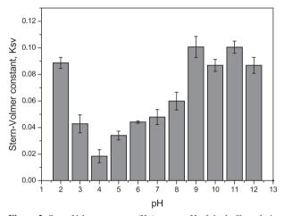
Figure 2. Stern-Volmer constant  $(K_{sv})$  versus pH of the buffer solution used to determination of quercetin. Buffer solution varied from 2 to 12.
