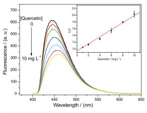
**Figure 4.** Fluorescence spectra for quercetin determination, reference solutions containing, 0; 1; 2; 4; 6; 8 and 10 mg  $L^{-1}$ , the insert is the analytical curve for quercetin.
