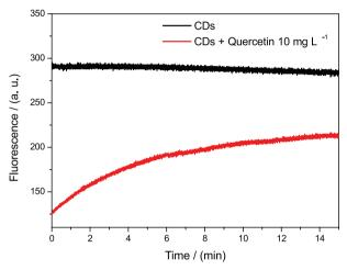
Figure 3. The transient signal for time of the reaction between carbon dot and quercetin (10 mg L<sup>1</sup>), pH 11. The signal was monitored at 450 nm.
