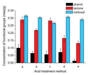
**Figure 7.** Potentiometric titration results of MWCNTs after OCF extraction for the samples submitted to treatments at: (a) 50 °C, 90 min and 176 mL; (b) 70 °C, 20 min and 176 mL; (c) 70 °C, 20 min and 88 mL; (d) 70 °C, 20 min and 44 mL; (e) 70 °C, 20 min and 20 mL.
