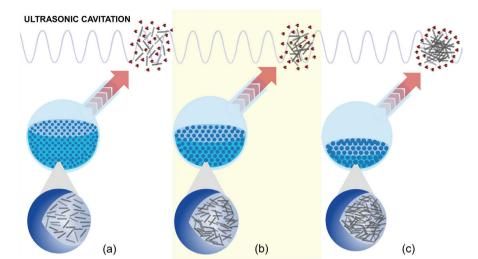
Figure 4. Illustrative scheme of ultrasonic cavitation influence on the functionalization of 3 g of MWCNTs with different acid volumes: (a) 176 mL, acid in excess; (b) 44 mL, optimal condition; (c) 20 mL, insufficient acid.
