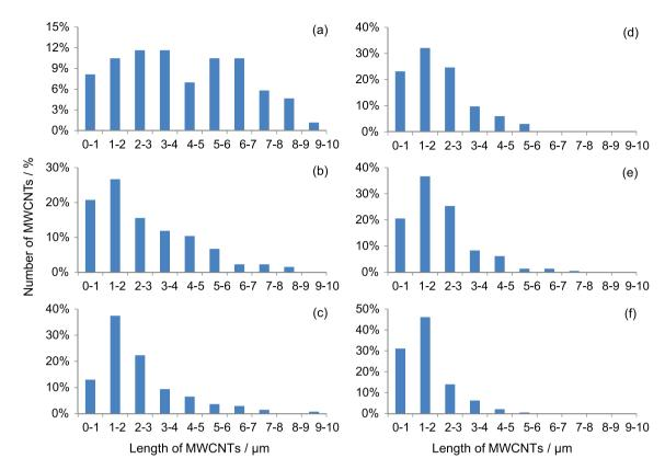
Figure 3. Length distribution of (a) pristine MWCNTs and modified MWCNTs after treatment at (b) 70 °C, 20 min and 20 mL; (c) 70 °C, 20 min and 44 mL; (d) 70 °C, 20 min and 88 mL; (e) 70 °C, 20 min and 176 mL; (f) 50 °C, 90 min and 176 mL.
