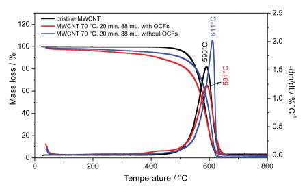
Figure 1. TGA analysis of MWCNTs treated at 70 °C, 20 min and 88 mL of acid, before and after OCF extraction.
