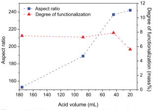
Figure 6. MWCNT aspect ratio and degree of functionalization as a function of acid volume for treatments at 70 °C and 20 min.
