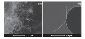
Figure 2. SEM images of (a) agglomerated MWCNTs and (b) isolated MWCNTs after functionalization at 70  $^{\circ}$ C, 20 min and 44 mL of acid volume.
