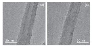
Figure 5. TEM images of (a) pristine MWCNTs and (b) functionalized MWCNTs at 70  $^{\circ}$ C, 20 min and 44 mL of acid volume.
