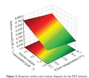
Figure 2. Response surface and contour diagram for the PET intrinsic viscosity assay.
