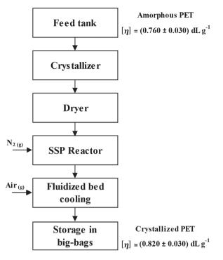
Figure 1. Simplified block diagram of the solid state polymerization (SSP) process of the recycled PET resin.
