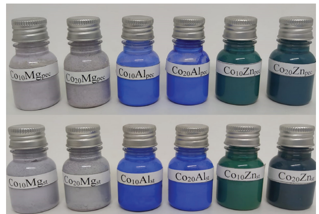
Figure 3. Photographs of Co-doping pigments in different host matrices (MgO, Al 2 O 3 , and ZnO) and different dopant concentrations.
