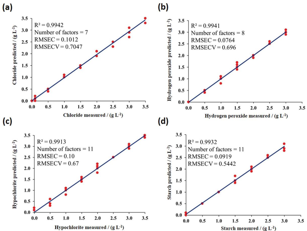
**Figure 3.** Correlation between the measured values and predicted values by PhotoMetrix UVC for chloride (a), hydrogen peroxide (b), hypochlorite (c), and starch (d) in raw milk samples with addition of analyte.
