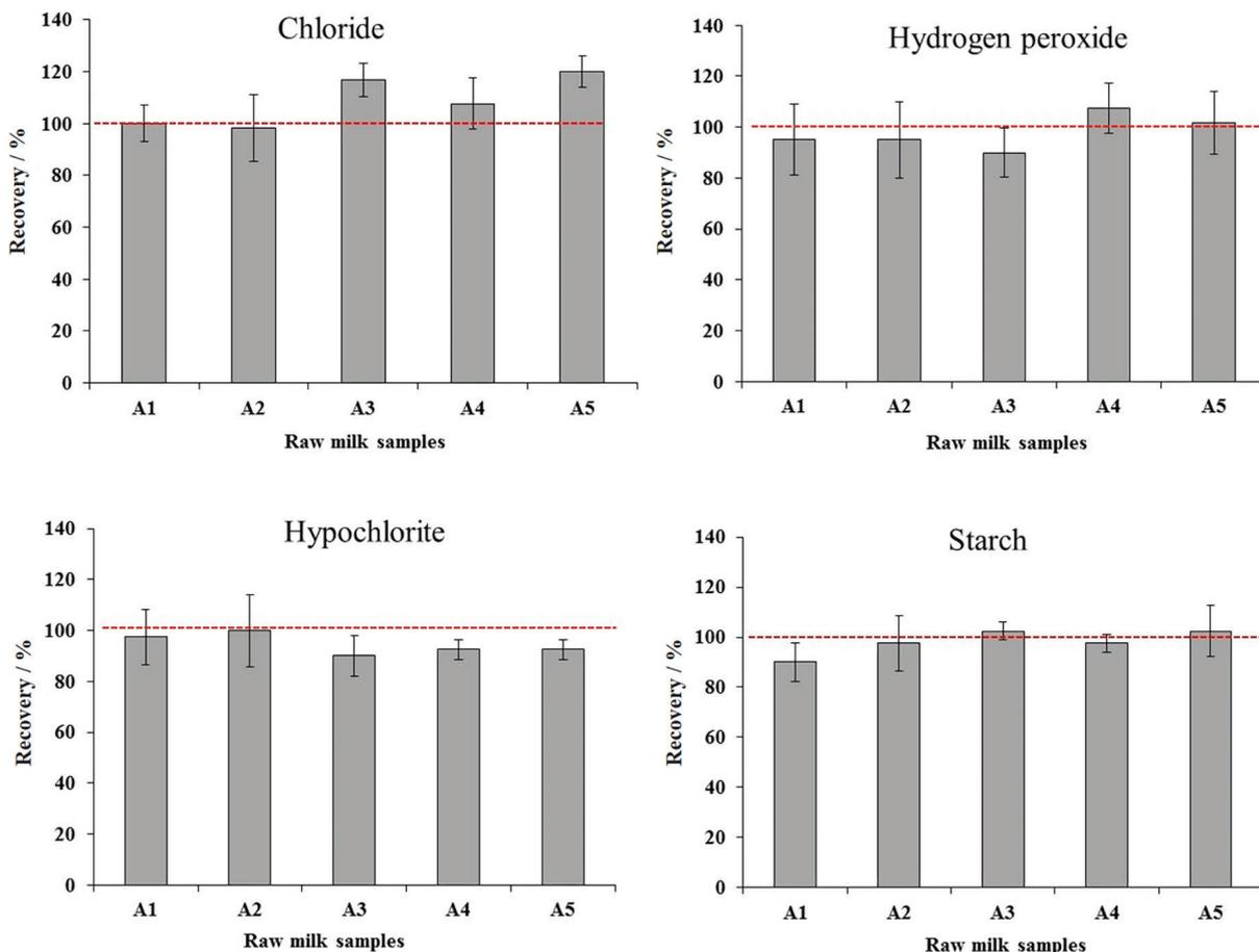
**Figure 4.** Recovery assays using PhotoMetrix UVC for chloride, hydrogen peroxide, hypochlorite, and starch added at concentrations of 2 g L<sup>-1</sup> (n = 3) in raw milk from five different cows.
