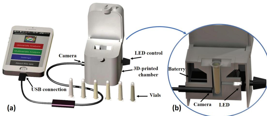
**Figure 1.** System used for colorimetric analysis using a UVC (a). Chamber details (b).
