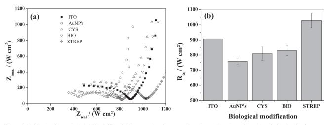
Figure 7. (a) Nyquist diagram in PBS (pH = 7.45) and (b) bar graph to charge transfer resistance for each working electrode functionalization steps. Amplitude used was 15 mV and frequency range was between 1 kHz and 10 mHz at -100 mV.
