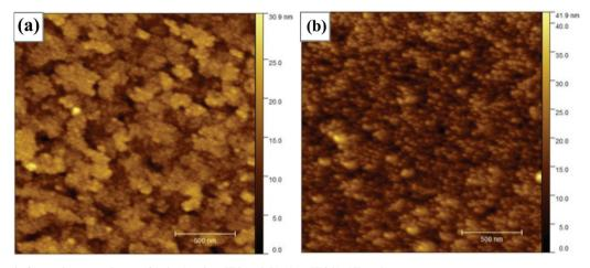
Figure 5. Atomic force microscopy images for the (a) glass-ITO and (b) glass-ITO/AuNPs substrates.
