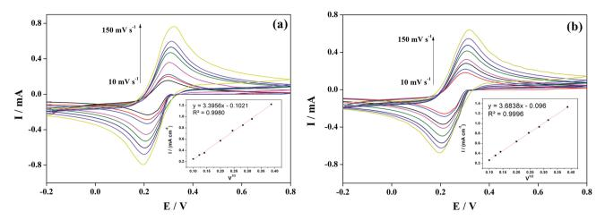
**Figure 4.** Cyclic voltammograms of  $K_3[Fe(CN)_6]$  (5.0 mmol L<sup>-1</sup>) in KCl (0.5 mol L<sup>-1</sup>) to the (a) glass-ITO and (b) glass-ITO/AuNPs substrates. Scanning rates were from 10 to 150 mV s<sup>-1</sup> (25 °C) and the anodic peak at 380 mV was evaluated. Insets show the current of the anodic peak *versus* square root of the scan rate.
