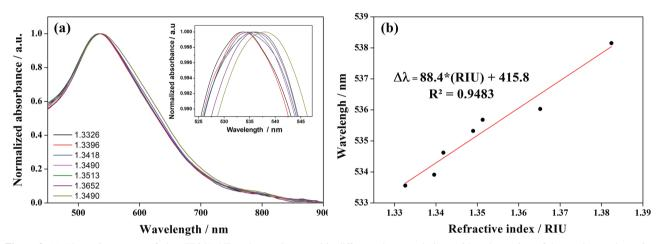
Figure 3. (a) Absorption spectra of glass-ITO/AuNPs substrate immersed in different glucose solutions with a closer view of the maximum absorption and (b) its linear fit with RI sensitivity of 88.4 nm RIU<sup>-1</sup>.
