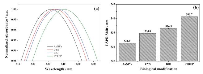
Figure 6. (a) Absorption spectra and (b) average  $\lambda_{max}$  for each functionalization steps of the biotest assay.
