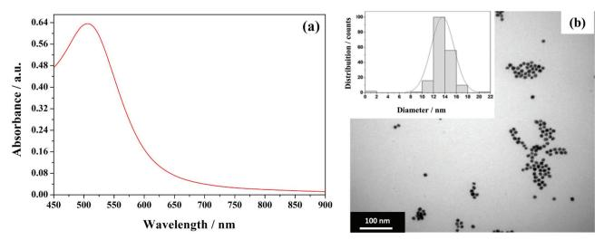
Figure 1. (a) Absorption spectra of AuNPs solution and (b) transmission electron microscopy image with a size distribution histogram.
