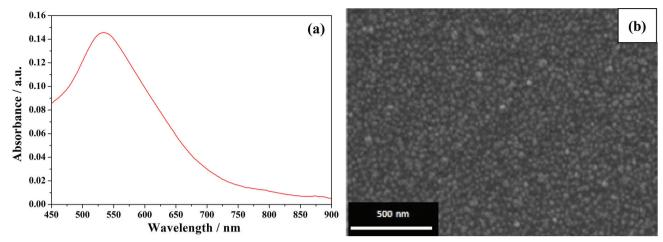
Figure 2. (a) Absorption spectrum and (b) scanning electron microscopy image of the AuNPs-coated glass-ITO substrates.
