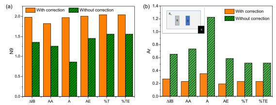
**Figure 3.** Parameters for each treatment applied to the experimental data for the red filters for the webcam, with and without white correction with the cuvette. (a) N9; (b) analytical resolution. Insert: schematic diagram of the constructed chamber.  $\Delta I_B$ : intensity variation (with white);  $A_A$ : absolute absorbance; A: absorbance;  $A_E$ : expanded absorbance; T: transmittance;  $T_E$ : expanded transmittance.
