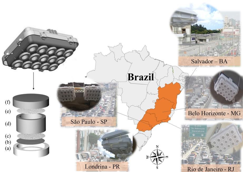
**Figure 1.** Representation of the location of the sampling stations and description of the passive sampler: (a) air inlet, (b) stainless steel mesh, (c) Teflon membrane, (d) diffusion space, (e) impregnated filter, (f) sampler bottom air inlet.
