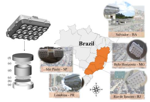
Figure 1. Representation of the location of the sampling stations and description of the passive sampler: (a) air inlet, (b) stainless steel mesh, (c) Teflon membrane, (d) diffusion space, (e) impregnated filter, (f) sampler bottom air inlet.
