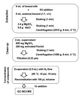
Figure 1. Sample preparation procedure for the determination of POPs and CUPs in breast milk.
