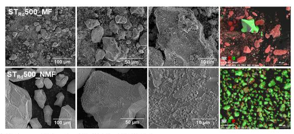
Figure 9. SEM images and EDS mapping of  $ST_{Rd}500\_MF$  and  $ST_{Rd}500\_NMF.$
