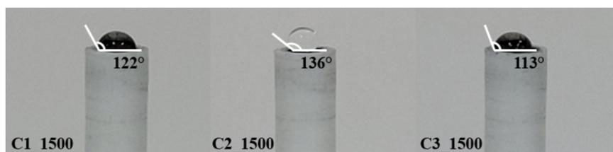
**Figure 8.** Profiles of water drop at surface of C1\_1500, C2\_1500 and C3\_1500 materials prepared in an 80:20 wt.% ratio (ceramic:Nujol®), compacted into a cavity electrode followed by polishing with paper flat surface and washing with ultrapure water.
