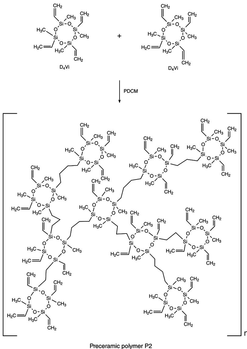
**Figure 2.** Schematic representation of the polymeric network P2, obtained by radical reaction among cyclic D<sub>4</sub>Vi molecules.
