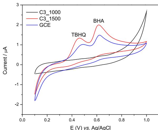
**Figure 7.** Cyclic voltammograms of TBHQ and BHA ethanol solution at  $0.1 \text{ mmol L}^{-1}$  concentration using C3\_1000, C3\_1500 and GCE in  $0.3 \text{ mol L}^{-1}$  BR buffer (pH 2.0) and scan rate of  $50 \text{ mV s}^{-1}$ .
