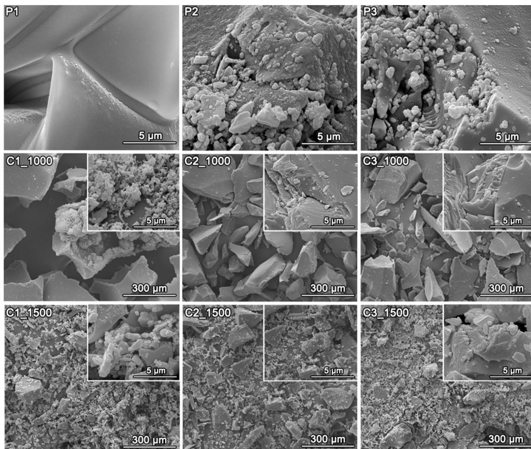
**Figure 6.** SEM images of preceramic polymers (P1, P2 and P3) and ceramic materials obtained at 1000 °C (C1\_1000, C2\_1000 and C3\_1000) and 1500 °C (C1\_1500, C2\_1500 and C3\_1500).
