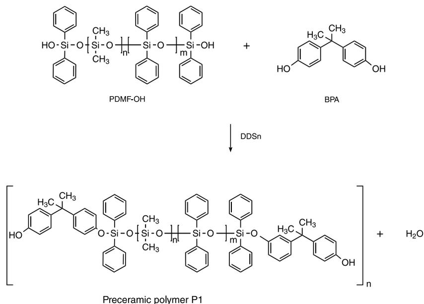
**Figure 1.** Schematic representation of the polymeric network P1, obtained by polycondensation reaction between linear PDMF-OH silicone and BPA organic crosslinker.
