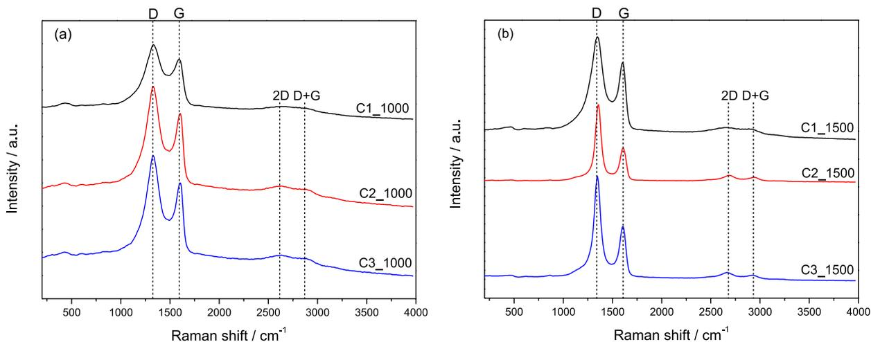
**Figure 5.** Raman spectra for C1, C2 and C3 ceramics obtained at 1000 °C (a) and 1500 °C (b).
