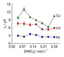
**Figure 2.** Peak currents for Cd, Pb and Cu as a function of  $HNO_3$  concentration in the ME. Biodiesel samples spiked with 12, 10 and 11 µg kg<sup>-1</sup> of Cd, Pb and Cu, respectively.
