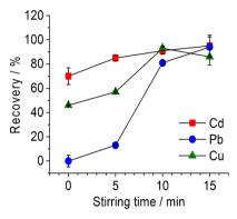
**Figure 3.** Recoveries for  $2.95 \,\mu g \, \text{kg}^{-1} \, \text{Cd}$ ,  $2.00 \,\mu g \, \text{kg}^{-1} \, \text{Pb}$  and  $2.40 \,\mu g \, \text{kg}^{-1} \, \text{Cu}$  in biodiesel with different stirring times during the EIMB. Stirring speed: 800 rpm.
