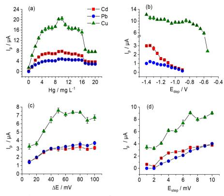
**Figure 4.** Peak currents of 50  $\mu$ g L<sup>-1</sup> Cd, Pb and Cu as a function of: (a) Hg<sup>II</sup> concentration, (b) E<sub>dep</sub>, (c)  $\Delta$ E and (d) E<sub>step</sub> in the solution in the cell containing the APE after EIMB. For (a) to (d): 2.30 mL APE and 2.70 mL of 1.0 mol L<sup>-1</sup> acetic acid/acetate buffer pH 4.6.
