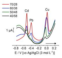
**Figure 1.** Square wave voltammograms in the APE after EIMB with ME containing different B/P ratios. Biodiesel samples spiked with 12, 10 and  $11 \ \mu g \ kg^{-1}$  of Cd, Pb and Cu, respectively.
