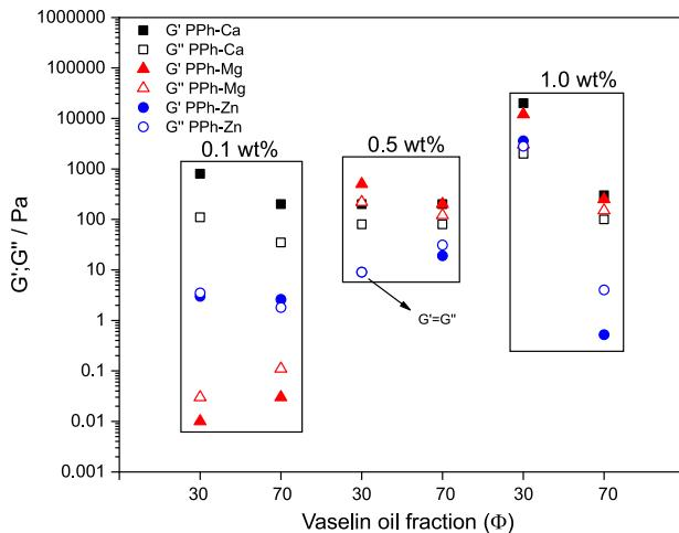
**Figure 5.** Rheological dynamic oscillatory analysis of emulsions stabilized with Ca-PPh, Zn-PPh and Mg-PPh with  $\Phi = 0.30$  or 30% and 0.70 or 70% in weight.
