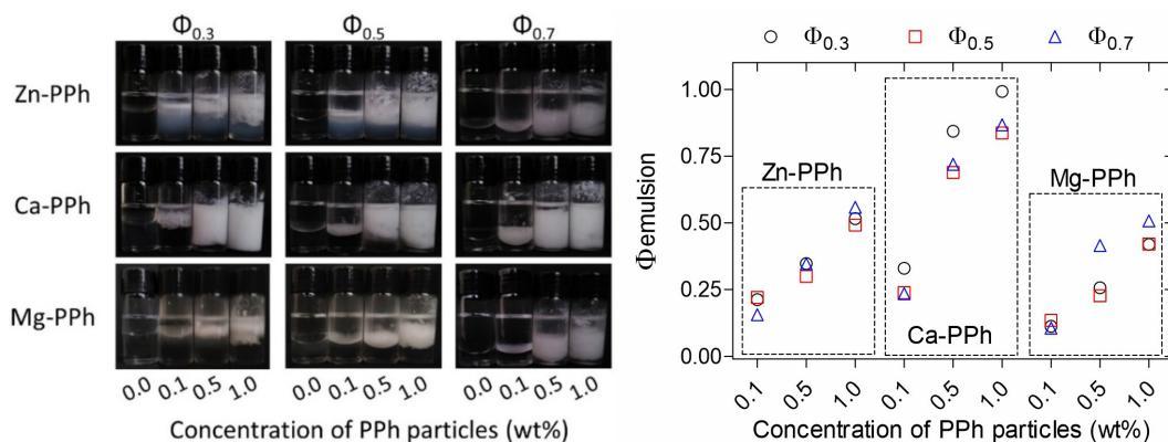
**Figure 4.** Emulsified portion ( $\Phi$ ) of the tubes 20 days after sonication with Ca-PPh, Zn-PPh and Mg-PPh particles in three different oil-in-water fractions (0.3, 0.5 and 0.7) and particle concentrations ranging from 0.1 to 1 wt.%.
