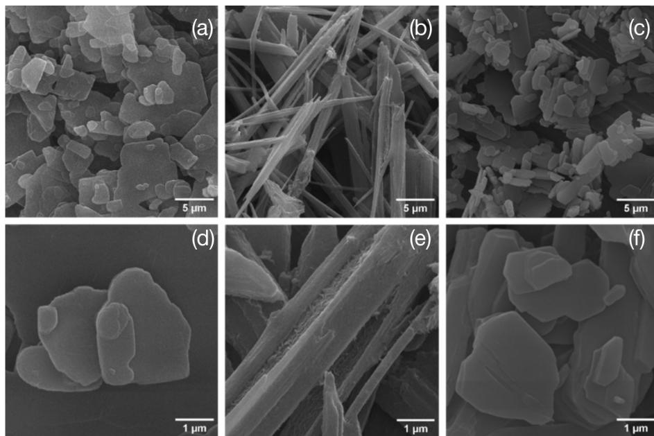
**Figure 3.** SEM images with magnifications of 10 and 50k $\times$ , respectively, of Zn-PPh (a, d), Ca-PPh (b, e), and Mg-PPh (c, f).
