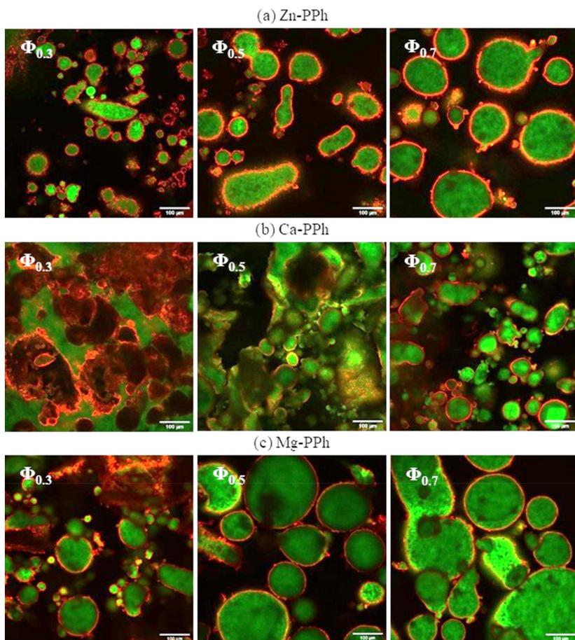
**Figure 7.** Confocal fluorescence microscopic image of emulsions containing oil and ultrapure water ( $\Phi_o$  ranging from 0.3–0.7) and 1.0 wt.% of particles of Zn-PPh (a), Ca-PPh (b) and Mg-PPh (c), 72 h after preparation (200 $\times$  magnification). The particles were stained with rhodamine B (2.5 ppm) and fluorescein (2.5 ppm) was used to stain the water. The scale bar is fixed at 100  $\mu\text{m}$ .
