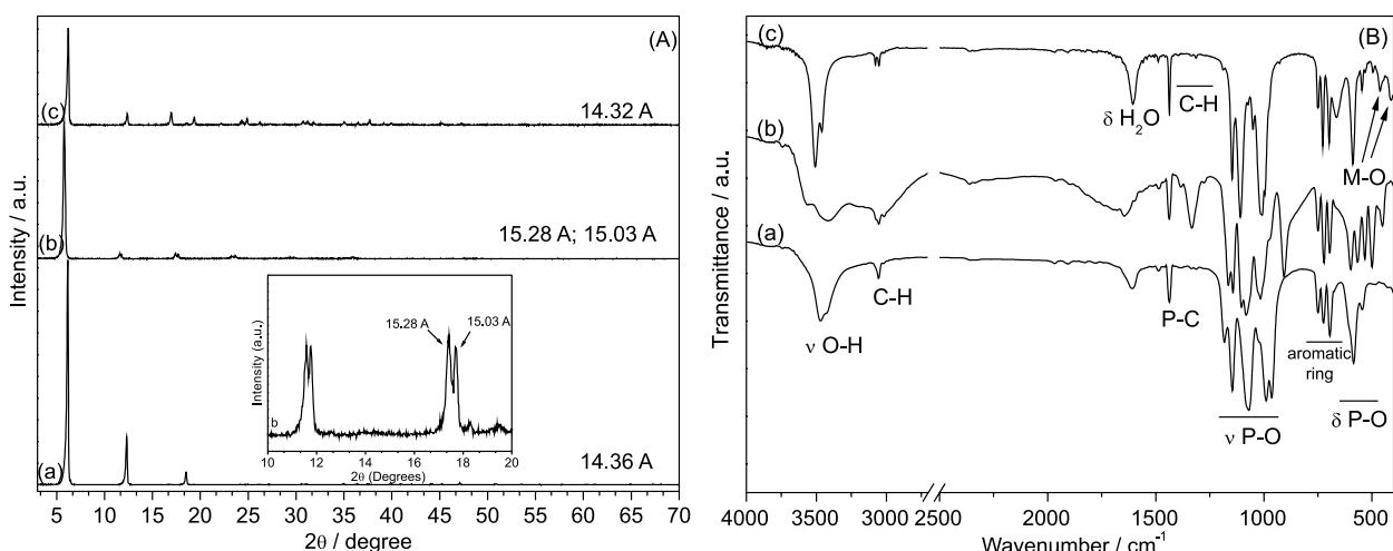
**Figure 2.** (A) XRD patterns and (B) FTIR (KBr) spectra of Zn-PPh (a), Ca-PPh (b), and Mg-PPh (c).
