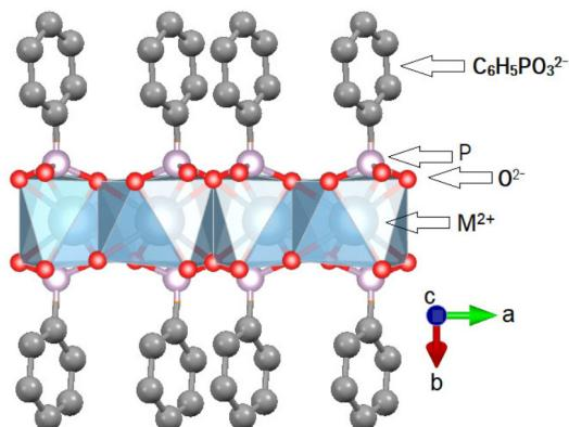
**Figure 1.** Schematic representation of a generic divalent metal phenylphosphonate structure oriented along the indicated axis.<sup>9</sup>
