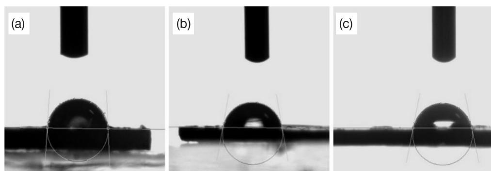
**Figure 6.** Contact angle measurements of droplets of water on pellets of hydrophobic Zn-PPh (a), Ca-PPh (b) and Mg-PPh (c).
