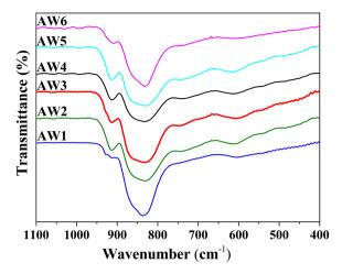
Figure 3. FTIR (KBr) spectra for the AW1, AW2, AW3, AW4, AW5 and AW6 samples prepared by the coprecipitation method at 25 °C for 3 h.
