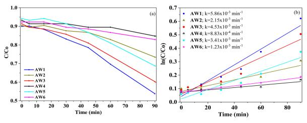
Figure 9. (a) Photocatalytic degradation of RhB for the AW1, AW2, AW3, AW4, AW5 and AW6 samples and (b) corresponding plot of ln (C\_/C) versus time.
