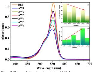
**Figure 8.** Photocatalytic tests on degradation of RhB dye in the presence AW1, AW2, AW3, AW4, AW5 and AW6 samples, using 50 mg of catalyst for 50 mL of solution of the dye, after 90 min of reaction. Insert (a) graph indicating the photocatalytic efficiency for the samples. (b) Graph indicating the average length of the crystals in the samples.
