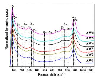
**Figure 4.** Raman spectra of AW1, AW2, AW3, AW4, AW5 and AW6 samples synthesized by coprecipitation method at 25 °C for 3 h. The vertical lines indicate the peak position of active modes.
