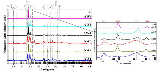
**Figure 2.** (a) X-ray diffraction patterns for the AW1, AW2, AW3, AW4, AW5 and AW6 samples prepared by the coprecipitation method at 25 °C for 3 h. The vertical lines indicate the peak position in the direction of each plane. (b) Enlarged view of the diffracted region between 28 and 33°.
