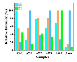
Figure 6. Graph of intensities relative to the (011), (001), (101) and (100) plans for AW1, AW2, AW3, AW4, AW5 and AW6 samples processed by the coprecipitation method at 25 °C for 3 h.
