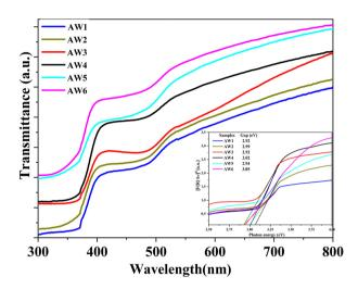
Figure 7. UV-Vis spectra of AW1, AW2, AW3, AW4, AW5 and AW6 and the inset shows direct band gap spectra obtained using the Kubelka-Munk method of the samples.
