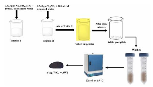
Figure 1. Scheme of synthesis of  $\alpha$ -Ag<sub>2</sub>WO<sub>4</sub> by coprecipitation method at 25 °C for 3 h.
