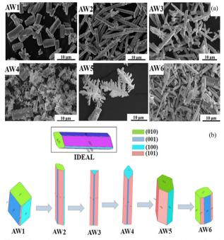
**Figure 5.** (a) SEM images for the AW1, AW2, AW3, AW4, AW5 and AW6 samples processed by the coprecipitation method at 25 °C for 3 h. (b) Illustrative scheme for the  $\alpha$ -Ag<sub>2</sub>WO<sub>4</sub> crystal with the crystallographic planes (010), (001), (100) and (101).
