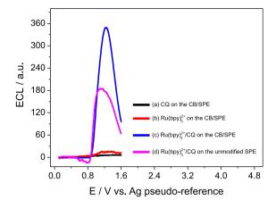
**Figure 2.** ECL-potential curves obtained for: (a) CB/SPE in CQ solution; (b) CB/SPE in Ru(bpy)<sub>3</sub><sup>2+</sup> solution; (c) CB/SPE in Ru(bpy)<sub>3</sub><sup>2+</sup>/CQ mixture; and (d) unmodified SPE in Ru(bpy)<sub>3</sub><sup>2+</sup>/CQ. Scan rate: 0.1 V s<sup>-1</sup>.
