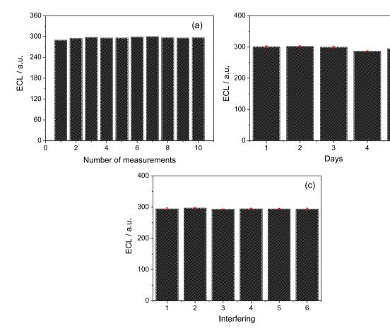
Figure 5. (a) ECL intensity measurements performed on the same working day and (b) on different days. Influence of possible interferences on the ECL signal strength for: (1) CQ + ascorbic acid; (2) CQ + citric acid; (3) CQ + glucose; (4) CQ + KCl; (5) CQ + NaCl; and (6) CQ + oflaxacin. The experiments were carried out in 0.1 mol L<sup>-1</sup> of phosphate buffer, pH 7.0.
