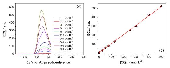
**Figure 4.** (a) ECL intensity for different CP concentrations (0-500  $\mu$ mol L<sup>-1</sup>). (b) Analytical curve obtained from the data in Figure 4a. [Ru(bpy)<sub>3</sub><sup>2+</sup>]: 5.0 mmol L<sup>-1</sup>. Scan rate: 0.1 V s<sup>-1</sup>.
