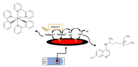
Scheme 1. Schematic representation of the electrochemiluminescent reaction between chloroquine and the ruthenium complex on the CB-modified SPE surface.
