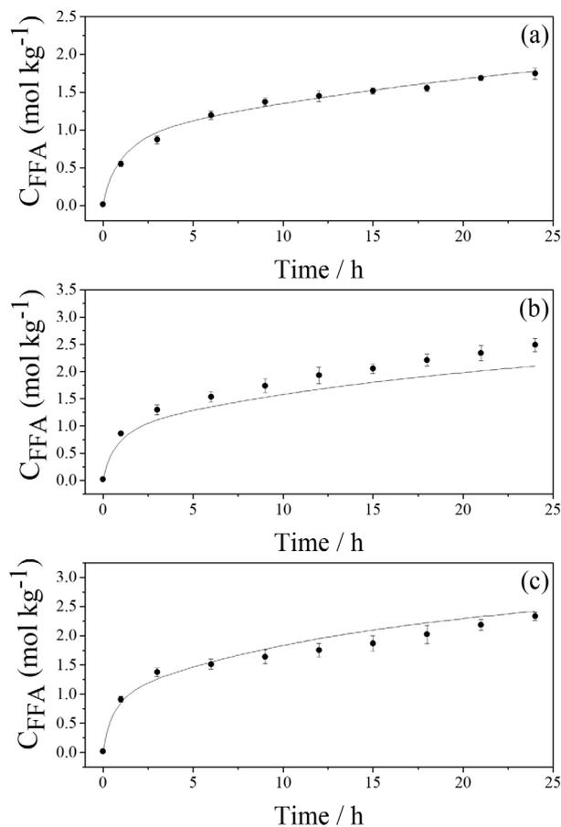
**Figure 7.** Prediction of the soybean oil enzymatic hydrolysis: (a) temperature 40 °C; (b) temperature 52 °C; (c) temperature 64 °C. Conditions: molar ratio W/O 20:1, enzyme/oil substrate ratio = 1% (m/m), stirring speed = 250 rpm; pH = 6.1. (●) Experimental data; (—) model.
