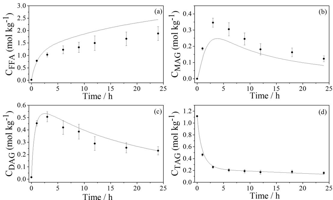
**Figure 3.** Simulation of the soybean oil enzymatic hydrolysis: (a)  $C_{\text{FFA}}$  ( $\text{mol kg}^{-1}$ ); (b)  $C_{\text{MAG}}$  ( $\text{mol kg}^{-1}$ ); (c)  $C_{\text{DAG}}$  ( $\text{mol kg}^{-1}$ ); (d)  $C_{\text{TAG}}$  ( $\text{mol kg}^{-1}$ ). Conditions: temperature = 40 °C; molar ratio W/O 46:1, enzyme/oil substrate ratio = 1% (m/m), stirring speed = 250 rpm; pH = 6.1. (●) Experimental data; (—) model.
