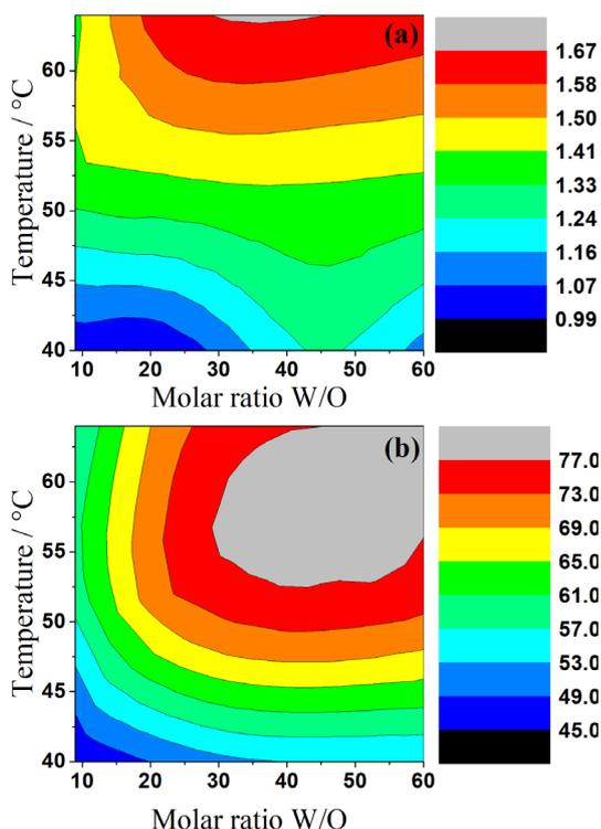
**Figure 2.** The initial reaction rate (a) and FFA yield (b). Experimental conditions: temperatures of 40, 52 and 64 °C, and molar ratios W/O of 9:1, 20:1, 46:1 and 60:1.
