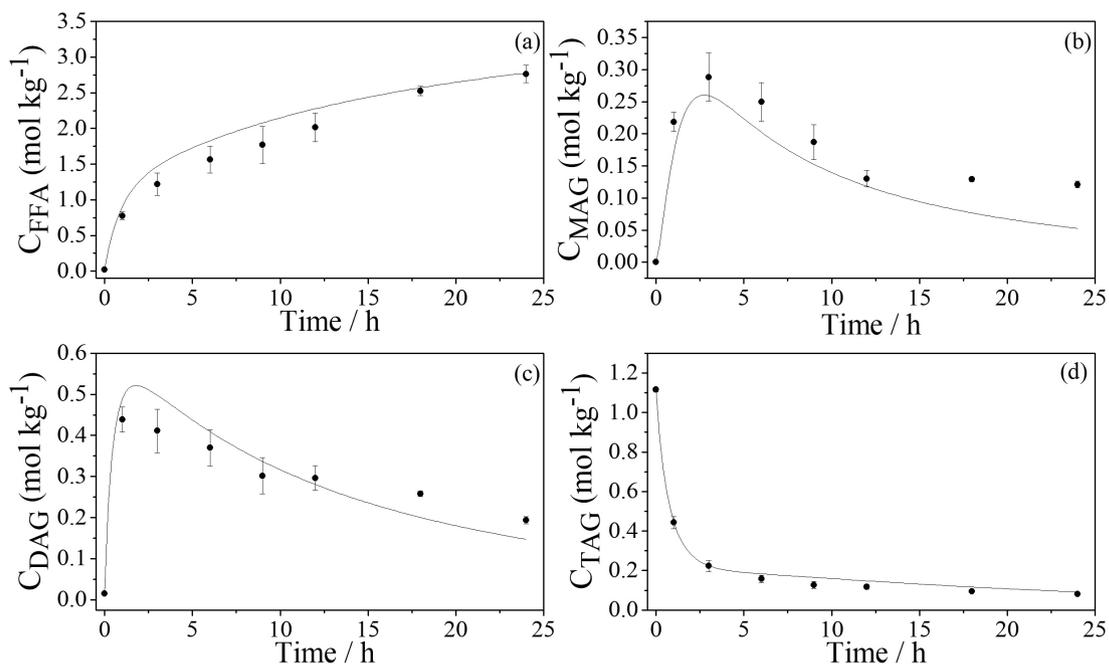
**Figure 4.** Simulation of the soybean oil enzymatic hydrolysis: (a)  $C_{\text{FFA}}$  ( $\text{mol kg}^{-1}$ ); (b)  $C_{\text{MAG}}$  ( $\text{mol kg}^{-1}$ ); (c)  $C_{\text{DAG}}$  ( $\text{mol kg}^{-1}$ ); (d)  $C_{\text{TAG}}$  ( $\text{mol kg}^{-1}$ ). Conditions: temperature = 52 °C; molar ratio W/O 46:1, enzyme/oil substrate ratio = 1% (m/m), stirring speed = 250 rpm; pH = 6.1. (●) Experimental data; (—) model.
