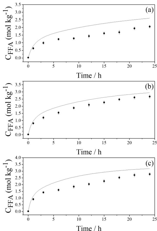
**Figure 8.** Prediction of the soybean oil enzymatic hydrolysis: (a) temperature 40 °C; (b) temperature 52 °C; (c) temperature 64 °C. Conditions: molar ratio W/O 60:1, enzyme/oil substrate ratio = 1% (m/m), stirring speed = 250 rpm; pH = 6.1. (●) Experimental data; (—) model.
