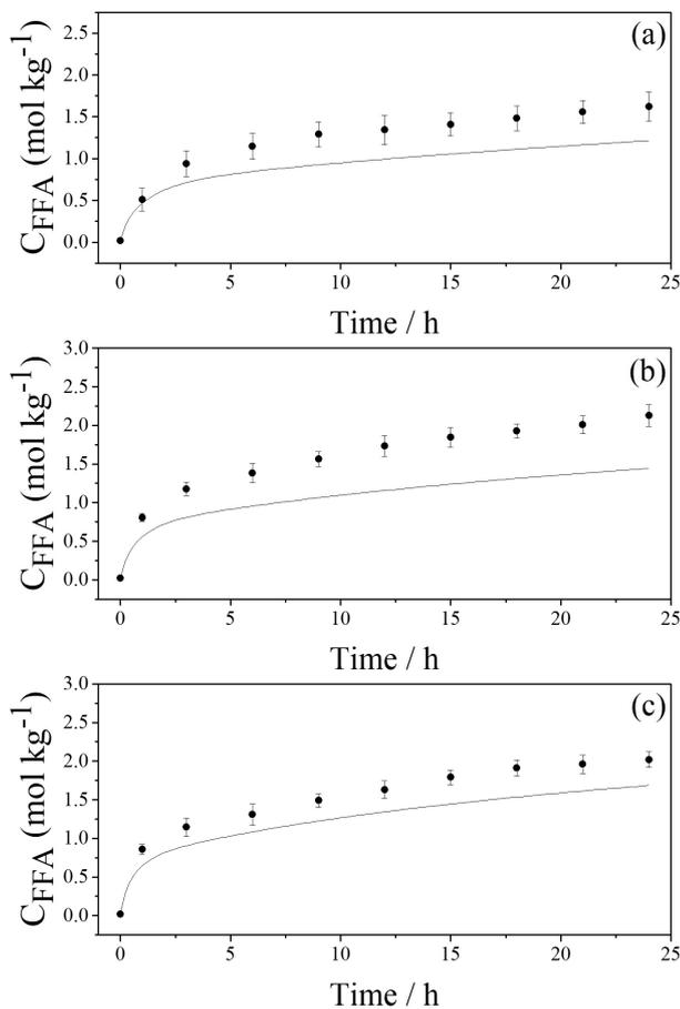
**Figure 6.** Prediction of the soybean oil enzymatic hydrolysis: (a) temperature 40 °C; (b) temperature 52 °C; (c) temperature 64 °C. Conditions: molar ratio W/O 9:1, enzyme/oil substrate ratio = 1% (m/m), stirring speed = 250 rpm; pH = 6.1. (●) Experimental data; (—) model.
