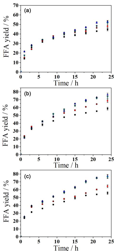
**Figure 1.** Kinetics of the soybean oil enzymatic hydrolysis for the molar ratios W/O of: 9:1 (■), 20:1 (●), 46:1 (▲), and 60:1 (▼). Experimental conditions: 250 rpm, molar ratio enzyme/oil 1% m/m, 40 °C (a), 52 °C (b) and 64 °C (c).
