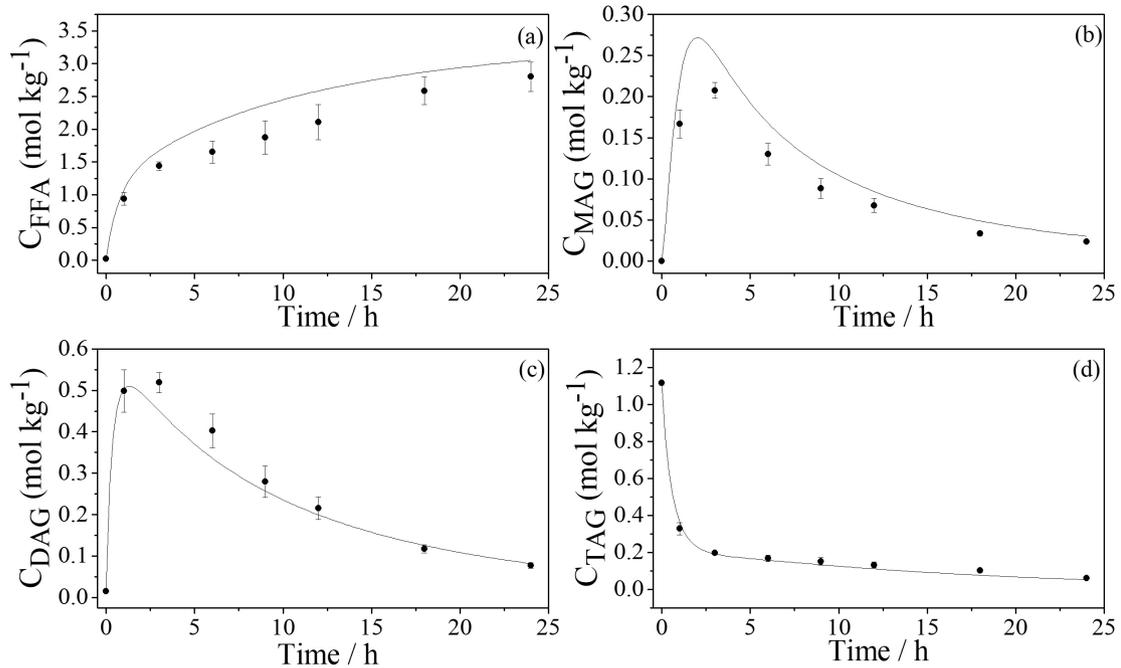
**Figure 5.** Simulation of the soybean oil enzymatic hydrolysis: (a)  $C_{\text{FFA}}$  ( $\text{mol kg}^{-1}$ ); (b)  $C_{\text{MAG}}$  ( $\text{mol kg}^{-1}$ ); (c)  $C_{\text{DAG}}$  ( $\text{mol kg}^{-1}$ ); (d)  $C_{\text{TAG}}$  ( $\text{mol kg}^{-1}$ ). Conditions: temperature = 64 °C; molar ratio W/O 46:1, enzyme/oil substrate ratio = 1% (m/m), stirring speed = 250 rpm; pH = 6.1. (●) Experimental data; (—) model.
