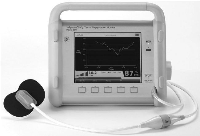
Figure 2 – An example of a near-infrared spectrophotometer (Inspectra, Hutchinson Technology Incorporated).
