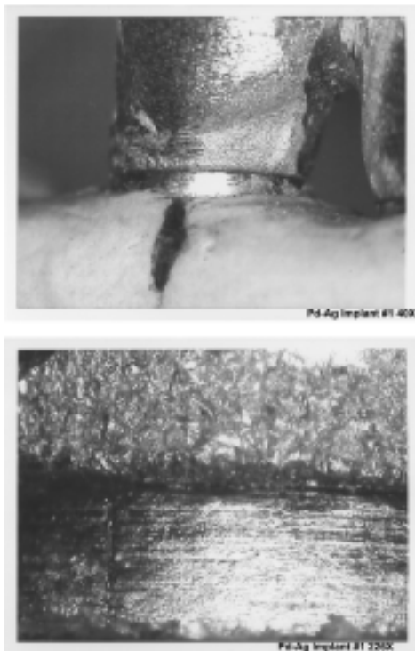
Figure 3. Pd-Ag alloy. Fit interfaces during Sheffield test of structure #1, implant #1. Magnification: top, 40X; bottom, 226X.
