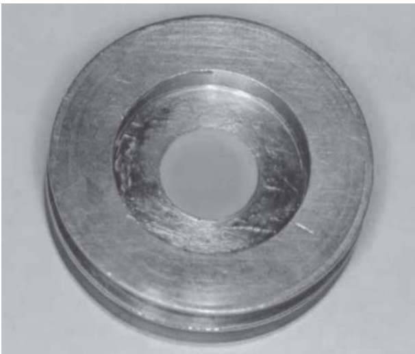
Figure 1. Stainless steel matrix with the test specimen. Upper view of the composite resin/adhesive system/composite resin setting.
