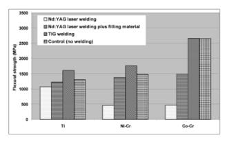
Figure 1. Flexural strength of the specimens samples displayed separated by material.
