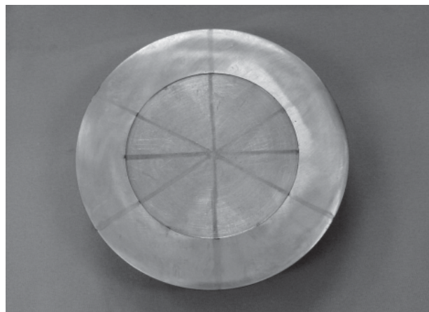
Figure 2. Cylindrical stainless steel support used for finishing procedures.
