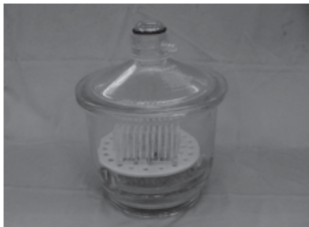
Figure 3. Recipient containing dry and fresh silica gel used during water sorption test.
