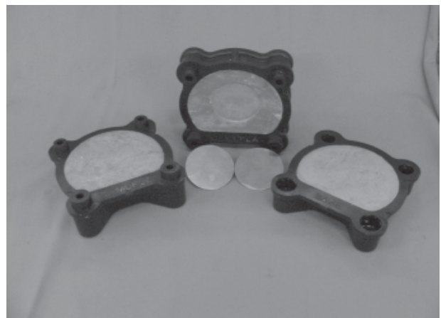
Figure 1. Polyvinyl chloride bimaxillary flasks used for polymerization in microwave oven.
