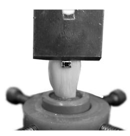
Figure 1. Bovine incisor with metallic bracket bonded to buccal enamel and the active chisel tip acting on the upper part of the bracket base during the shear bond strength test.
