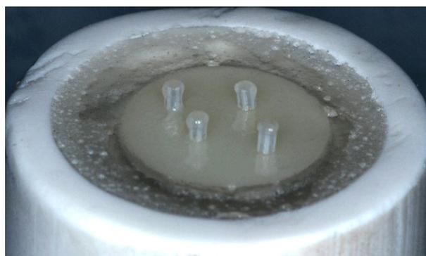
Figure 1. Positioning of Tygons on the ceramic discs surface.
