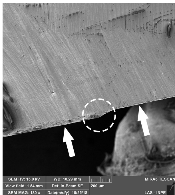
Figure 5. FEG-SEM micrograph (180x magnification) showing the interface between worn and non-worn areas of glazed specimen. It is possible to observe that the glaze layer was removed after the wear, but still a thin layer is present (arrows).
