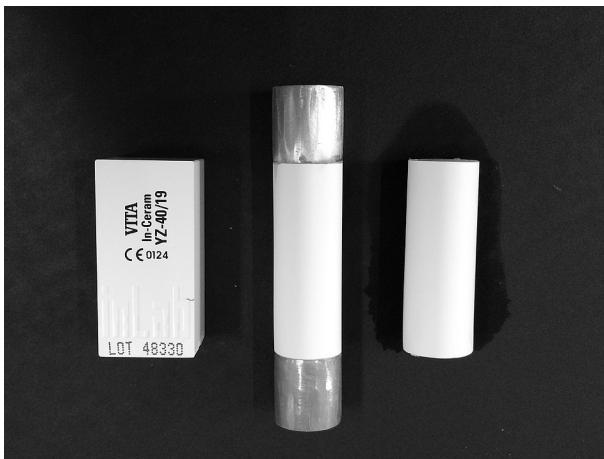
Figure 1. Zirconia cylinder: a block (A) was glued to a round index (B) and rounded until reaching the desired format and dimensions (C).
