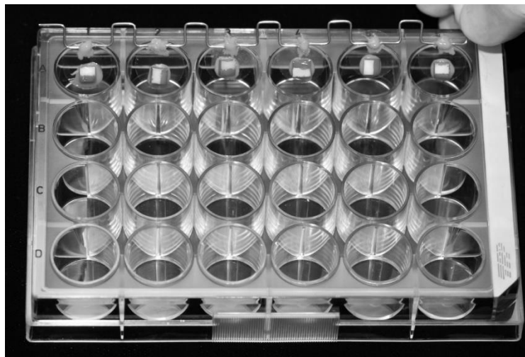
Figure 2. System used to maintain the samples individually suspended in a 24-well culture plate during the artificial caries lesion development.
