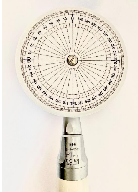
Figure 1. The 5-cm Polypropylene disk with registration from 0° - 360° with intervals at each degree used in the experiment
