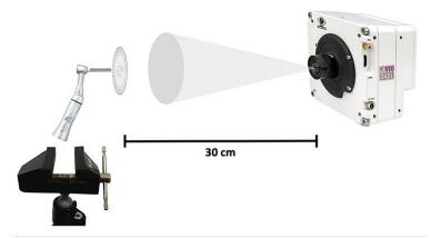
**Figure 2.** Apparatus for image acquisition – a set consisting of a camera, lenses, the target object and handpiece.
