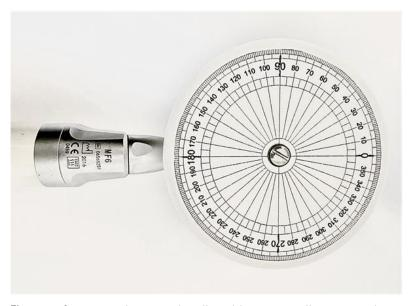
**Figure 1.** Custom angle-measuring disc with a 50-mm diameter used as a target object.
