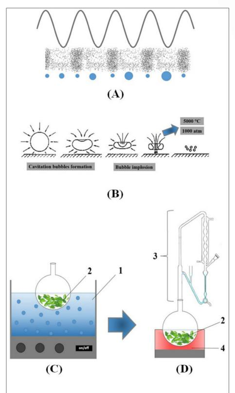
Figure 1 - A) Cavitation bubbles formation. B) Cavitation effect observed in the ultrasound. Adapted from VAN WIJNGAARDEN, 2016. C) System of pretreatment using ultrasound bath. D) Hydrodistillation before pretreatment. 1 – ultrasound bath, 2 - water with sample, 3 - distillation system, 4 - heating.
