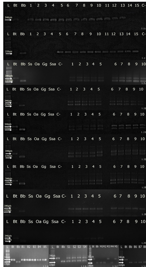
Figure 1 - 1.5% agarose gel showing the presence of cattle (346 bp) and buffalo (220 bp) DNA.
