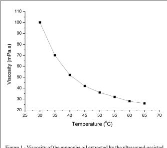
Figure 1 - Viscosity of the munguba oil extracted by the ultrasound-assisted method versus temperature increase.
