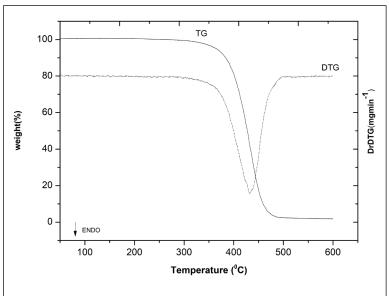
Figure 2 - Thermogravimetry and derivative thermogravimetry curves of munguba oil extracted by the ultrasound-assisted extraction method.
