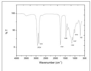
Figure 4 - Fourier-transform infrared spectrum of the munguba oil extracted by the ultrasound-assisted extraction method.
