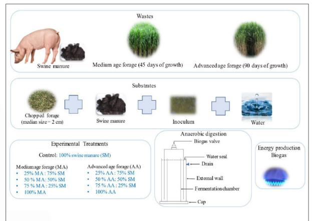
Figure 1 - Representation of the anaerobic co-digestion process of swine manure with different grass inclusions at two harvesting ages.
