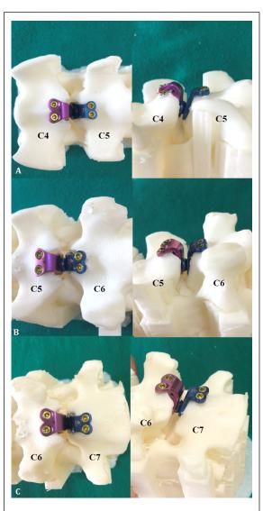
Figure 8 - Picture showing the ventral and lateral aspects of the third generation of the PVTM Cervical Disc prosthesis machined in titanium and implanted into the intervertebral spaces of (A) C4-C5; (B) C5-C6, and (C) C6-C7.
