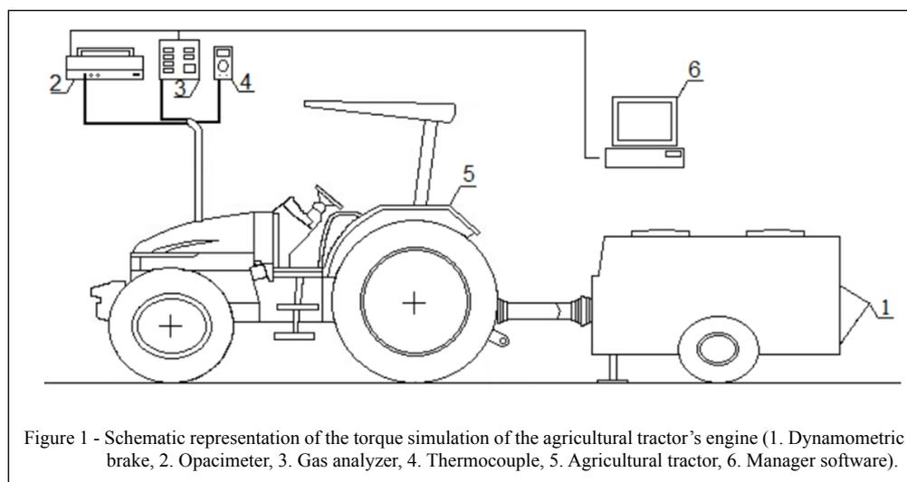
We obtained the gas opacity values using an EGGERS Opacilyt ELD partial-flow opacimeter.
